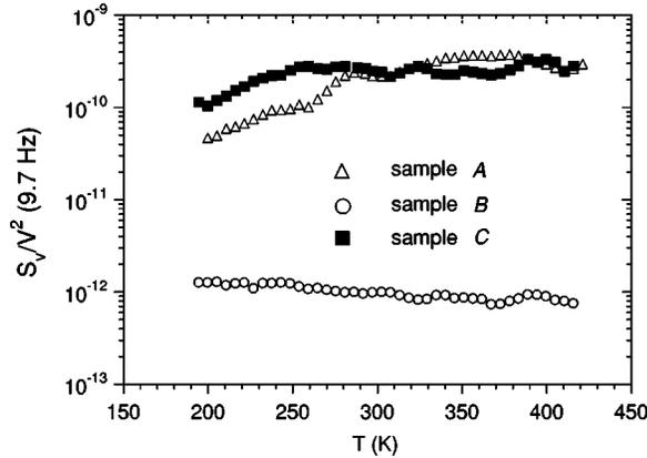
FIG. 3. The normalized noise power at 9.7 Hz as a function of temperature ( $200 \text{ K} \leq T \leq 430 \text{ K}$ ) for the three diamond samples. Insulating samples A and C, in which hopping conduction processes are important, show similar behavior with  $T$  while the just-metallic sample B shows quite different behavior.
