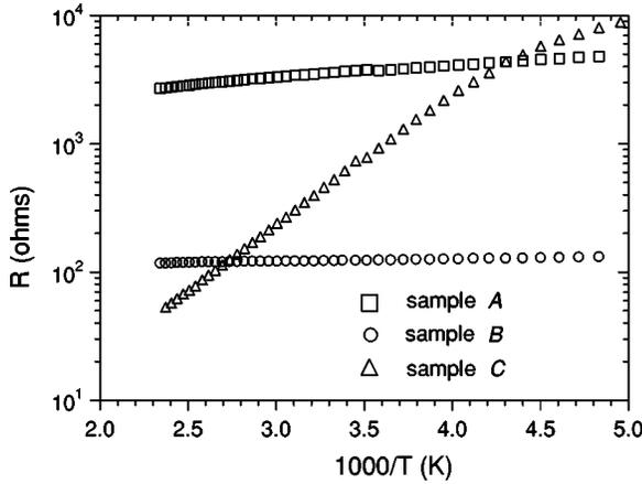
FIG. 1. Resistance versus  $1000/T$  ( $200 \text{ K} \leq T \leq 430 \text{ K}$ ), for three boron-doped diamond samples. Sample A ( $0.6 \times 10^{21} \text{ cm}^{-3}$ ), and sample B ( $4.1 \times 10^{21} \text{ cm}^{-3}$ ) are boron-implanted single crystals. Sample C ( $\sim 1 \times 10^{18} \text{ cm}^{-3}$ ) is boron-doped polycrystalline CVD diamond.
