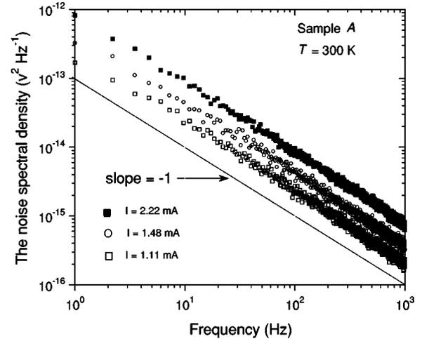
FIG. 2. The  $1/f$  noise spectral density as a function of frequency and dc current for boron-implanted diamond sample A at room temperature.
