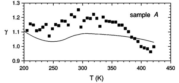
FIG. 4. The  $1/f$  noise spectral slopes  $\gamma$  vs temperature ( $200 \text{ K} \leq T \leq 430 \text{ K}$ ) for boron-implanted diamond sample A. The solid curve is the prediction of the DDH model (Ref. 15) given in Eq. (2).
