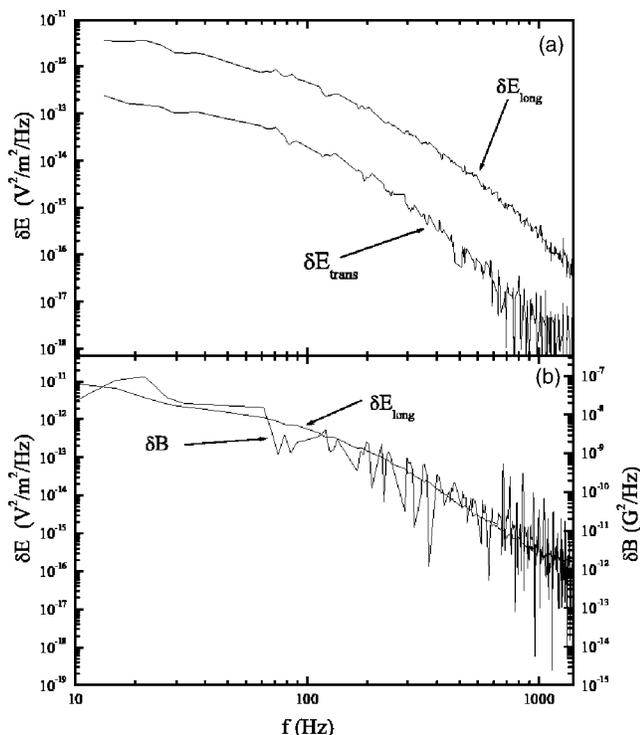
FIG. 5. Up: Longitudinal and transverse electric fields noise spectra. Down: Longitudinal electric-field noise and magnetic-field noise spectra. Both are taken in flux flow ( $B=0.23$  T,  $T=4.2$  K,  $I=6.9$  A). Note the similarity of the shape for all the spectra.
