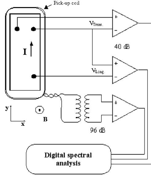
FIG. 1. Electric-field and magnetic-field noise experimental setup. The current is supplied by batteries and yields noise-free currents. All amplifying equipments are electromagnetically shielded.
