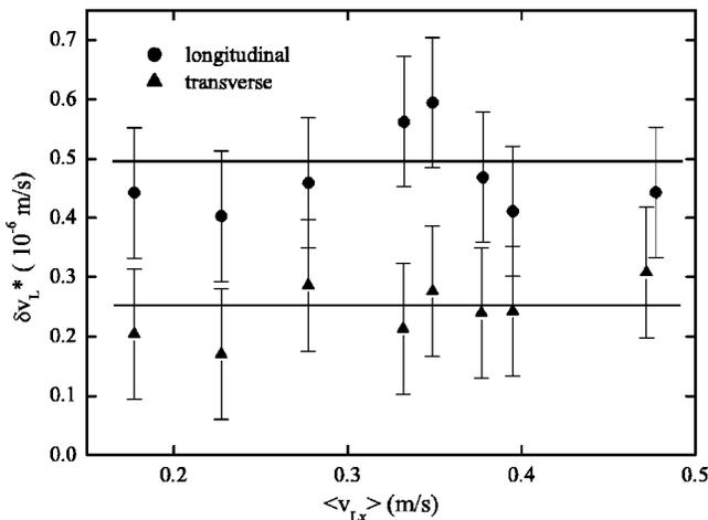
FIG. 4. Velocity fluctuations in the longitudinal ( $\bullet$ ) and transverse ( $\blacktriangle$ ) directions plotted against the mean velocity of the lattice  $\langle v_{Lx} \rangle$  ( $T=4.2$  K,  $B=0.1$  T). This range of velocities corresponds to the flux-flow regime. Dotted lines are guides for the eyes.
