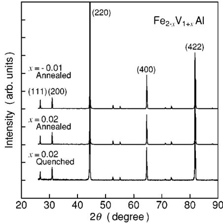
FIG. 1. Powder x-ray diffraction patterns for  $\text{Fe}_{2-x}\text{V}_{1+x}\text{Al}$ : the annealed  $x=-0.01$  sample, and the  $x=0.02$  samples annealed and quenched after holding at 1173 K, respectively.
