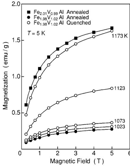
FIG. 8. Magnetic-field dependence of magnetization measured at 5 K in  $\text{Fe}_{2.01}\text{V}_{0.99}\text{Al}$  ( $x=-0.01$ ) and  $\text{Fe}_{1.98}\text{V}_{1.02}\text{Al}$  ( $x=0.02$ ). The solid and open symbols show the data on annealed and quenched samples, respectively.
