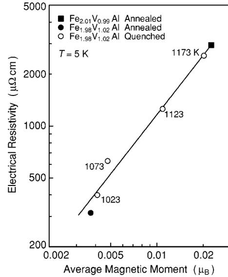
FIG. 9. Relation between the electrical resistivity at 5 K and the average magnetic moment of Fe atoms in  $\text{Fe}_{2.01}\text{V}_{0.99}\text{Al}$  ( $x=-0.01$ ) and  $\text{Fe}_{1.98}\text{V}_{1.02}\text{Al}$  ( $x=0.02$ ). The solid and open symbols show the data on annealed and quenched samples, respectively.
