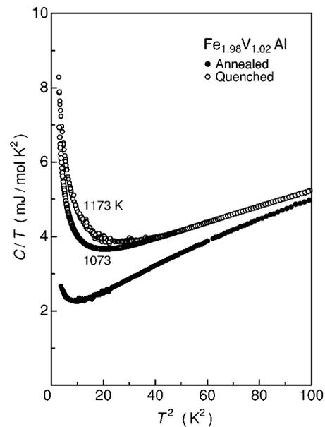
FIG. 6. The specific heat over temperature,  $C/T$ , vs  $T^2$  measured for  $\text{Fe}_{1.98}\text{V}_{1.02}\text{Al}$  ( $x=0.02$ ) quenched after holding at 1173 and 1073 K (open circles): the solid circles show the data on the annealed sample.
