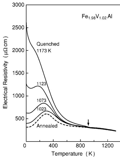
FIG. 5. Temperature dependence of electrical resistivity in  $\text{Fe}_{1.98}\text{V}_{1.02}\text{Al}$  ( $x=0.02$ ) quenched after holding at 1173, 1123, 1073, and 1023 K: the dotted curve is for the annealed sample. The arrow shows the inflection of the resistivity curves.
