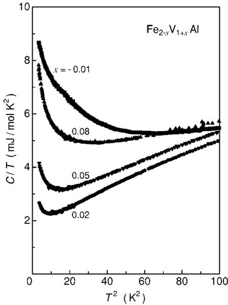
FIG. 4. Specific heat over temperature,  $C/T$ , vs  $T^2$  measured for  $\text{Fe}_{2-x}\text{V}_{1+x}\text{Al}$  with compositions  $-0.01 \leq x \leq 0.08$ .
