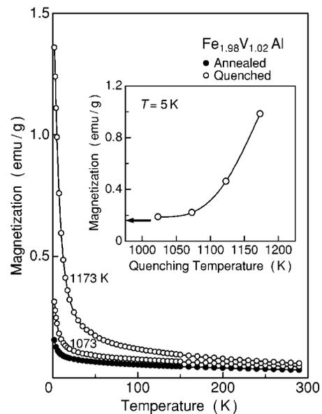
FIG. 7. Temperature dependence of magnetization in  $\text{Fe}_{1.98}\text{V}_{1.02}\text{Al}$  ( $x=0.02$ ) quenched after holding at 1173 and 1073 K (open circles): the solid circles show the data on the annealed sample. The magnetization was measured under a magnetic field of 1 T. The inset shows the magnetization at 5 K as a function of quenching temperature: the arrow indicates the value for the annealed sample.
