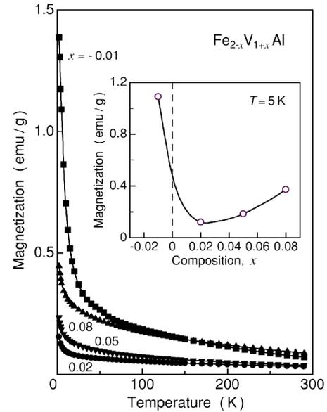
FIG. 2. Temperature dependence of magnetization in  $\text{Fe}_{2-x}\text{V}_{1+x}\text{Al}$  with compositions  $-0.01 \leq x \leq 0.08$ . The magnetization was measured under a magnetic field of 1 T. The inset shows the magnetization at 5 K as a function of composition  $x$ .
