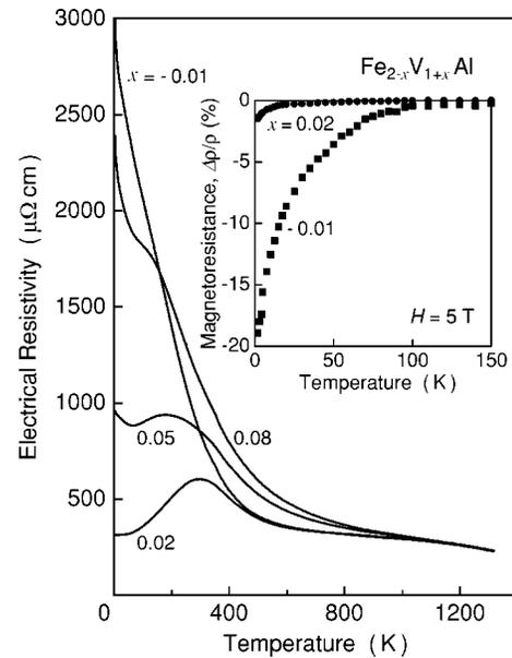
FIG. 3. Temperature dependence of electrical resistivity in  $\text{Fe}_{2-x}\text{V}_{1+x}\text{Al}$  with compositions  $-0.01 \leq x \leq 0.08$ . The inset shows the temperature dependence of the magnetoconductance  $\Delta\rho/\rho$  measured under 5 T magnetic field for  $x=-0.01$  and 0.02.
