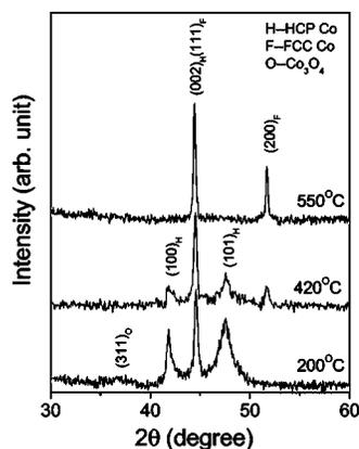
FIG. 7. X-ray diffraction patterns of Co particles prepared by the reduction of CoO nanoparticles at 200 °C, 420 °C, and 550 °C, respectively.
