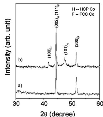
FIG. 8. X-ray diffraction profiles of the Co particles after a 3 h and 550 °C annealing of hcp nanoparticles by laser pyrolysis at 350 °C, (a) without and (b) with a gentle grinding during the XRD specimen preparation.
