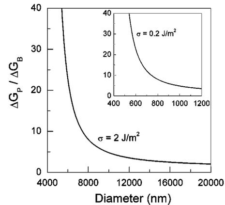
FIG. 9. The calculated generalized activation energy for martensitic transformation as a function of the diameter of Co particles at the surface energy of 2 J/m<sup>2</sup> and 0.2 J/m<sup>2</sup>.
