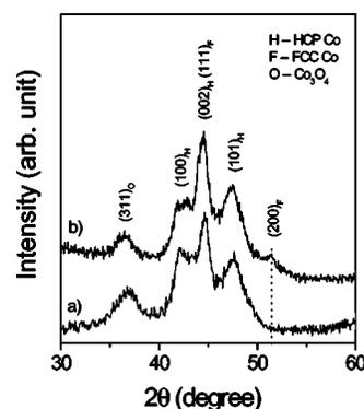
FIG. 2. X-ray diffraction patterns of Co nanoparticles prepared by laser pyrolysis: (a) at 325 °C and (b) at 427 °C, respectively.
