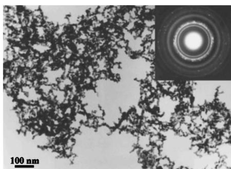
FIG. 3. Electron micrograph and corresponding selected area diffraction patterns of the hcp Co nanoparticles prepared at 325 °C.
