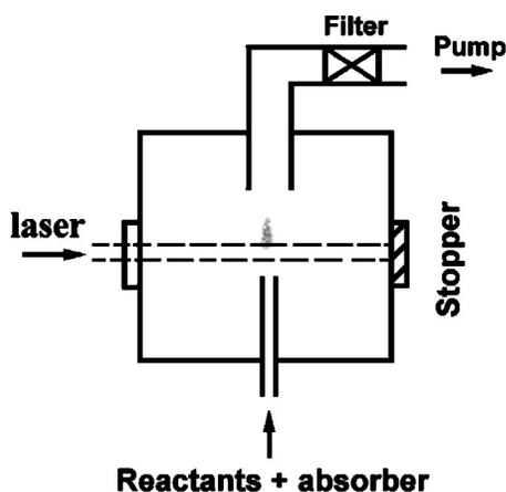
FIG. 1. Schematic representation of laser-induced pyrolysis.
