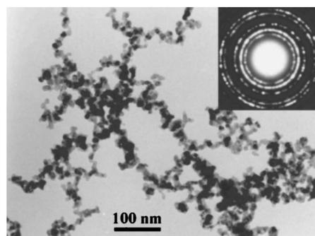
FIG. 4. Electron micrograph and corresponding selected area diffraction patterns of the CoO nanoparticles by laser pyrolysis.
