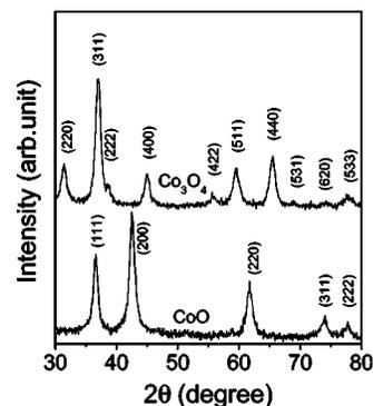
FIG. 5. X-ray diffraction patterns of CoO nanoparticles by laser pyrolysis and  $\text{Co}_3\text{O}_4$  nanoparticles by reduction of the CoO precursor.
