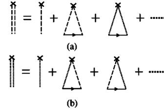
FIG. 2. Diagrams for (a) the  $T$  matrix (double dashed line) and (b) the  $\tilde{T}$  matrix (double dotted line). The single-dashed and single-dotted lines with crosses represent, respectively,  $V\tau_0$  and  $V\tau_2$ . The solid lines with arrows denote the impurity-averaged Green's function matrices.
