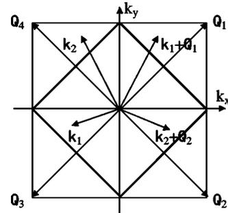
FIG. 1. Brillouin zone for the DDW state. The area enclosed by the heavy lines is the *reduced* Brillouin zone.  $Q_i$  ( $i=1, 2, 3, 4$ ) denote the nesting vectors.
