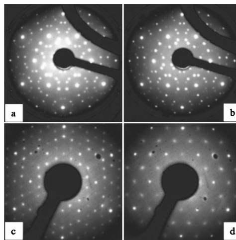
FIG. 1. K- and Cs-induced LEED patterns on  $\text{Ag/Si(111)}\sqrt{3} \times \sqrt{3}$ . (a)  $\sqrt{21} \times \sqrt{21}$ -K at 100 K, 64 eV. (b)  $\sqrt{21} \times \sqrt{21}$ -Cs at 100 K, 64 eV. (c)  $6 \times 6$ -K surface at RT, 61 eV; (d)  $2\sqrt{3} \times 2\sqrt{3}$ -K at RT, 63 eV.
