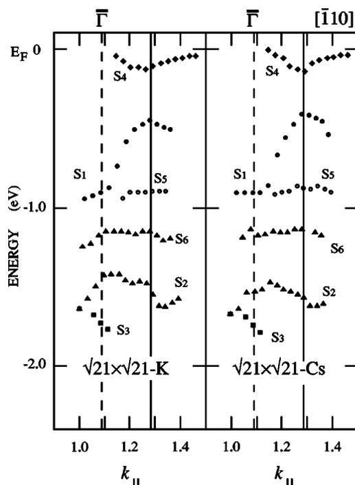
FIG. 4. Dispersions of the surface state bands along the  $\bar{\Gamma}$ - $\bar{M}$ - $\bar{\Gamma}$  line of the  $\sqrt{3}\times\sqrt{3}$  SBZ from Fig. 2. (a)  $\sqrt{21}\times\sqrt{21}$ -K. (b)  $\sqrt{21}\times\sqrt{21}$ -Cs. The dashed lines indicate the second  $\bar{\Gamma}$  point of the  $\sqrt{3}\times\sqrt{3}$  SBZ. The solid lines indicate the  $\sqrt{21}\times\sqrt{21}$  SBZ boundary.
