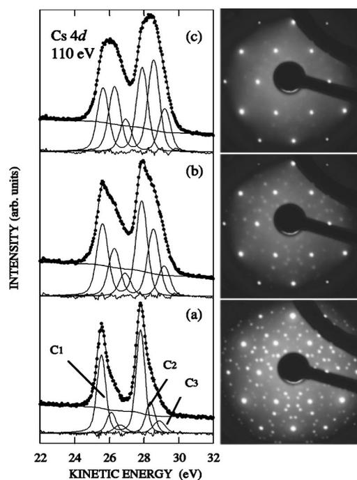
FIG. 5. Cs 4d core-level spectra recorded with a photon energy of 110 eV at normal emission and corresponding LEED patterns (96 eV) at 100 K. (a) Cs was evaporated for 6 min. (b) Cs was evaporated for 12 min. (c) Cs was evaporated for 18 min. A spin-orbit splitting of 2.26 eV, a branching ratio of  $\sim 0.7$ , and a singularity index of 0.02 were used in the fitting program. The two small components, C2 and C3, are shifted by 0.6 and 1.1 eV with respect to C1.
