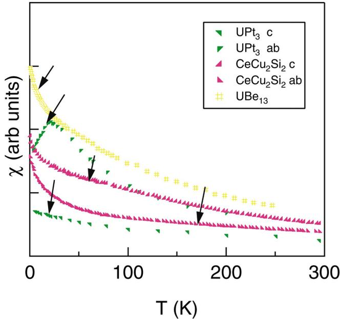
FIG. 18. (Color) The susceptibility  $\chi$  versus temperature in UPt<sub>3</sub>, CeCu<sub>2</sub>Si<sub>2</sub>, and UBe<sub>13</sub>.  $T^*$  is marked with an arrow.
