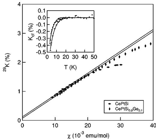
FIG. 10. The Si Knight shift in  $\text{CePtSi}_{1-x}\text{Ge}_x$  for  $x=0.0$  and  $x=0.1$  versus the bulk susceptibility.<sup>25</sup> The solid lines are fits to the high temperature data. Inset:  $K_{cf}$  versus  $T$ , and a fit to Eq. (8).
