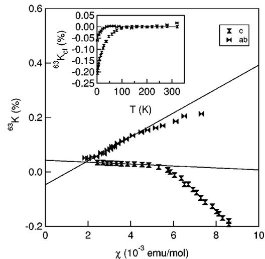
FIG. 8. The Cu Knight shift in CeCu<sub>2</sub>Si<sub>2</sub> versus the bulk susceptibility.<sup>13</sup> The solid lines are fits to the high temperature data. Inset:  $K_{cf}$  versus  $T$ , and a fit to Eq. (8).
