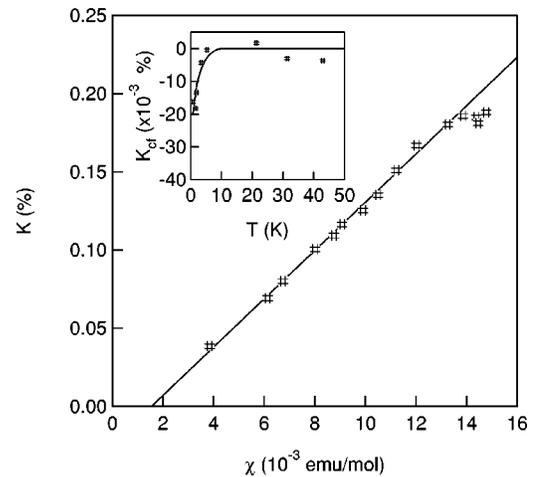
FIG. 15. The Be Knight shift in  $\text{UBe}_{13}$  versus the bulk susceptibility.<sup>40</sup> The solid line is a fit to the high temperature data. Inset:  $K_{cf}$  versus  $T$ , and a fit to Eq. (8).
