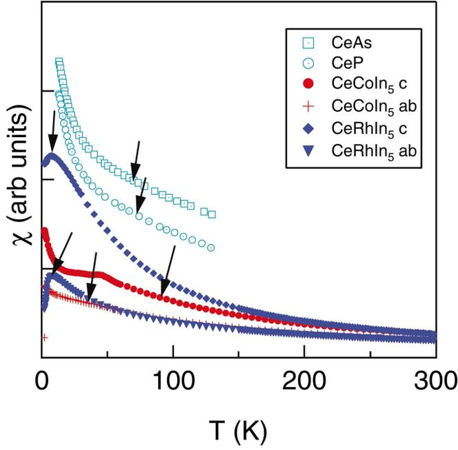
FIG. 17. (Color) The susceptibility  $\chi$  versus temperature in CeAs, CeP, CeCoIn<sub>5</sub>, and CeRhIn<sub>5</sub>.  $T^*$  is marked with an arrow. The data for CeAs and CeP are offset vertically for clarity.
