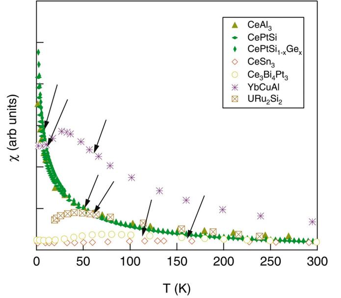
FIG. 19. (Color) The susceptibility  $\chi$  versus temperature in CeAl<sub>3</sub>, CePtSi<sub>1-x</sub>Ge<sub>x</sub>, CeSn<sub>3</sub>, Ce<sub>3</sub>Bi<sub>4</sub>Pt<sub>3</sub>, YbCuAl, and URu<sub>2</sub>Si<sub>2</sub>.  $T^*$  is marked with an arrow.
