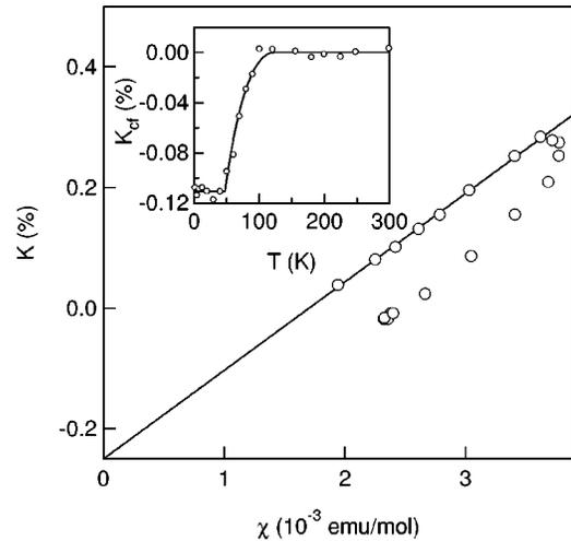
FIG. 11. The Bi Knight shift  $\text{Ce}_3\text{Bi}_4\text{Pt}_3$  versus the bulk susceptibility.<sup>30</sup> The solid line is a fit to the high temperature data. Inset:  $K_{cf}$  versus  $T$ , and a fit to Eq. (8).
