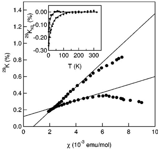
FIG. 9. The Si Knight shift in  $\text{CeCu}_2\text{Si}_2$  versus the bulk susceptibility.<sup>13</sup> The solid lines are fits to the high temperature data. Inset:  $K_{cf}$  versus  $T$ , and a fit to Eq. (8).
