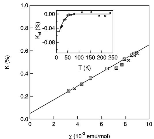
FIG. 16. The Si Knight shift in  $\text{URu}_2\text{Si}_2$  versus the bulk susceptibility.<sup>34</sup> The solid line is a fit to the high temperature data. Inset:  $K_{cf}$  versus  $T$ , and a fit to Eq. (8).
