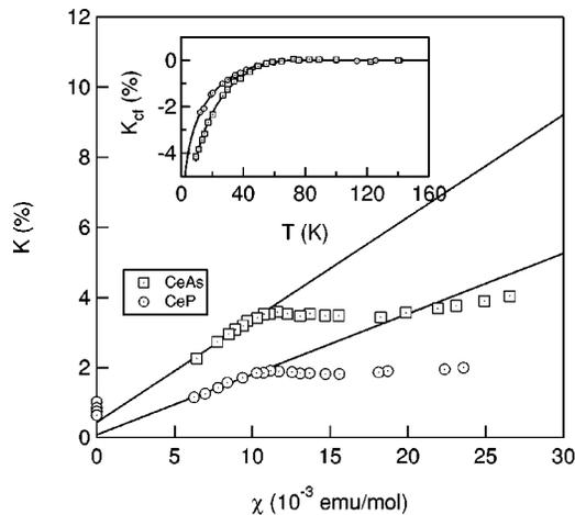
FIG. 13. The P and As Knight shifts in CeP and CeAs versus the bulk susceptibility.<sup>11</sup> The solid line is a fit to the high temperature data. Inset:  $K_{cf}$  versus  $T$ , and a fit to Eq. (8).
