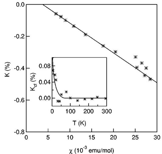
FIG. 12. The Cu Knight shift in  $\text{YbCuAl}$  versus the bulk susceptibility.<sup>32</sup> The solid line is a fit to the high temperature data. Inset:  $K_{cf}$  versus  $T$ , and a fit to Eq. (8).
