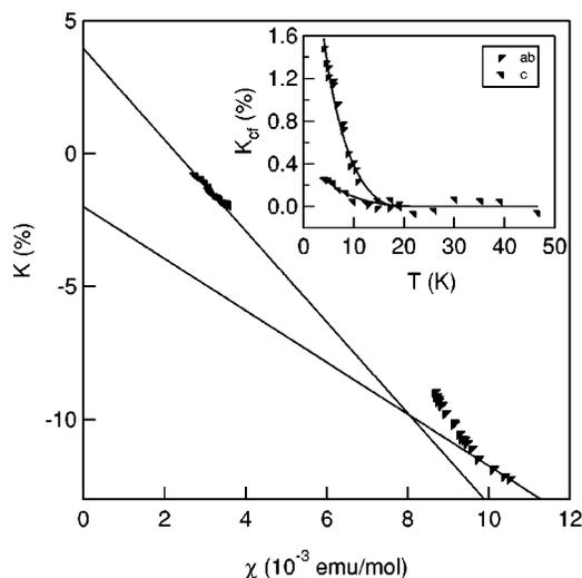
FIG. 14. The Pt Knight shift in  $\text{UPt}_3$  versus the bulk susceptibility.<sup>38,50</sup> The solid line is a fit to the high temperature data. Inset:  $K_{cf}$  versus  $T$ , and a fit to Eq. (8).
