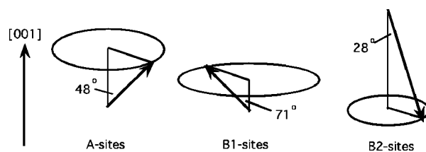
FIG. 4. Mean ferrimagnetic spiral order of \text{CoCr}_2\text{O}_4 estimated by the present neutron scattering experiments.
