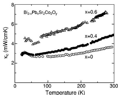
FIG. 3. Out-of-plane thermal conductivity of  $\text{Bi}_{2-x}\text{Pb}_x\text{Sr}_2\text{Co}_2\text{O}_y$ .
