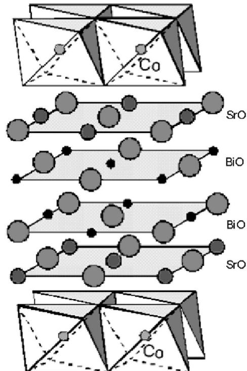
FIG. 1. Crystal structure of  $\text{Bi}_{2-x}\text{Pb}_x\text{Sr}_2\text{Co}_2\text{O}_y$ .
