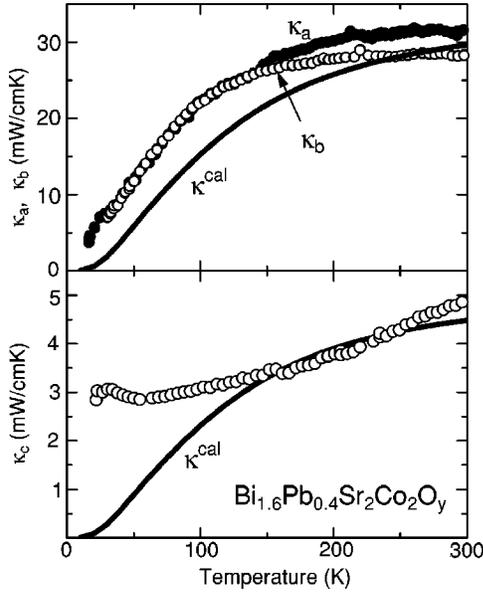
FIG. 4. Anisotropic thermal conductivity of  $\text{Bi}_{1.6}\text{Pb}_{0.4}\text{Sr}_2\text{Co}_2\text{O}_y$ .
