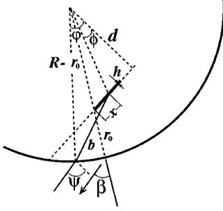
FIG. 1. Schematic illustration of a circular microdisk of a radius  $R$  with a linear defect. The defect position is characterized by  $r_0$ —the distance from the defect edge to the disk circumference along the radius; the defect orientation is fixed by the minimal distance,  $d$ , from the defect line to the disk center. The direction of the outgoing light is characterized by the angle  $\beta$  measured from the line connecting the edge of the defect to the center of the disk.
