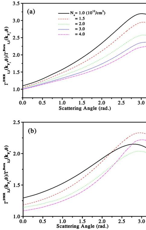
FIG. 1. The ratio of the scattering rates obtained within the LS equation and the Born approximation for conduction electrons in (a) the first and (b) the second subbands for the  $\delta$ -doped systems with different densities.
