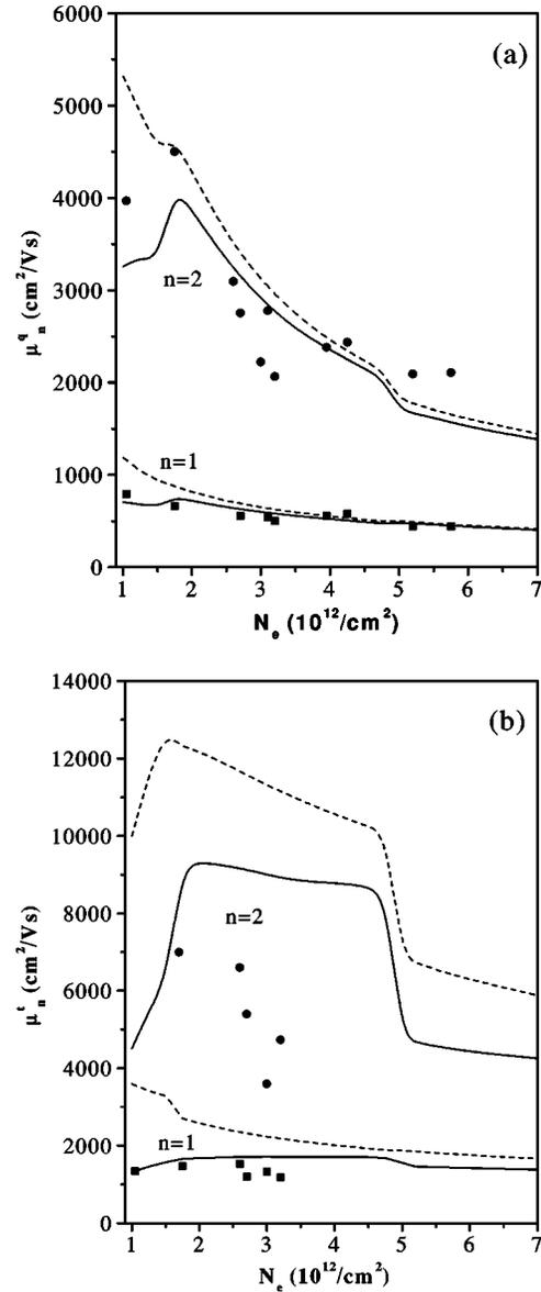
FIG. 2. (a) The quantum and (b) the transport mobilities for the first ( $n=1$ ) and second ( $n=2$ ) subbands in the  $\delta$ -doped system. The solid and dashed curves are obtained within the LS equation and the Born approximation, respectively. The experimental mobilities are indicated by the symbols.
