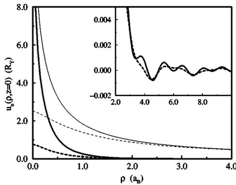
FIG. 3. The bare (thin curves) and screened (thick curves) impurity potential at the  $z=0$  plane in the real space for electrons in the first (solid curves) and the second (dashed curves) subbands.  $N_e=10^{12}$  cm $^{-2}$ ,  $R_y=5.48$  meV,  $a_B=99.8$  Å,  $E_{F1}=25.50$  meV, and  $E_{F2}=4.18$  meV. The inset shows the Friedel oscillations.
