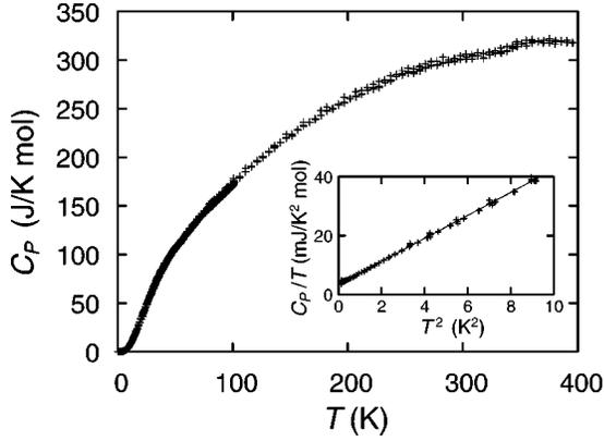
FIG. 4. Specific heat of  $\text{Ag}_5\text{Pb}_2\text{O}_6$  down to 0.35 K. These figures contain the results of several different samples. Inset:  $C_p/T$  plotted against  $T^2$  below 3.3 K. Solid line is the fitting  $C_p(T)/T = \gamma_e + \beta_p T^2$  with  $\gamma_e = 3.42 \text{ mJ/K}^2 \text{ mol}$  and  $\beta_p = 3.91 \text{ mJ/K}^4 \text{ mol}$ .
