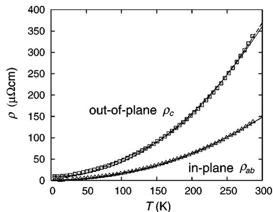
FIG. 3. Temperature dependence of the out-of-plane (open squares) and the in-plane resistivity (open triangles) down to 3 K. Solid lines are the fitting with  $\rho(T)=\rho_0+A'T^p$  with  $p=2.13$  for  $\rho_c$  and  $p=2.11$  for  $\rho_{ab}$ . Dashed lines are the fitting assuming the existence of an Einstein-like optic phonon mode.
