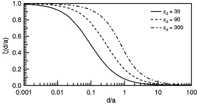
FIG. 2. Function  $\xi(d/a)$  versus the fraction  $d/a$  for three values of the passive layer permittivity  $\varepsilon_d$ ;  $\varepsilon_a, \varepsilon_c=300$ .
