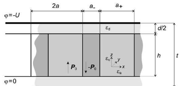
FIG. 1. Schema of the electroded ferroelectric film with passive layers. It is always considered that  $h \gg d$ .
