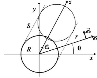
FIG. 2. Cylindrical model of the ferromagnetic nanotube.
