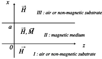
FIG. 1. Thin film representation of the ferromagnetic nanotube.
