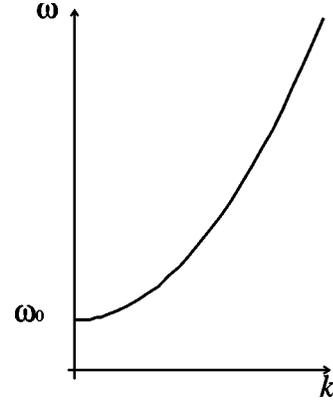
FIG. 3. The dispersion relation for MSW in hollow nanotubes.
