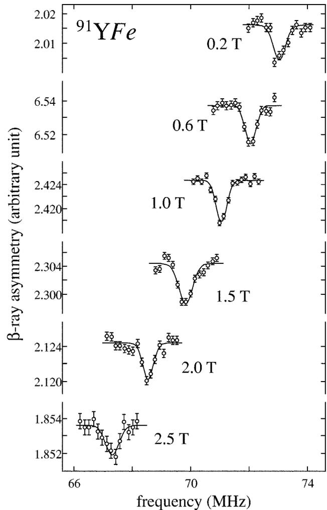
FIG. 1. Beta-NMRON spectra of  $^{91}\text{Y}$  in Fe for external applied fields of 0.2, 0.6, 1.0, 1.5, 2.0, and 2.5 T. The solid lines are results of the fit the data point to a Gaussian function.
