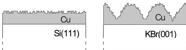
FIG. 1. Sketch of the two types of Cu films that are investigated in this work: mesoscopically smooth films on Si and mesoscopically rough films on KBr. Due to the same growth temperature the same adsorption properties are expected for the surfaces of these films.
