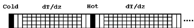
FIG. 1. Molecular dynamics setup for calculating the thermal conductivity of a straight carbon nanotube. The ellipses indicate that periodic boundary conditions are applied.
