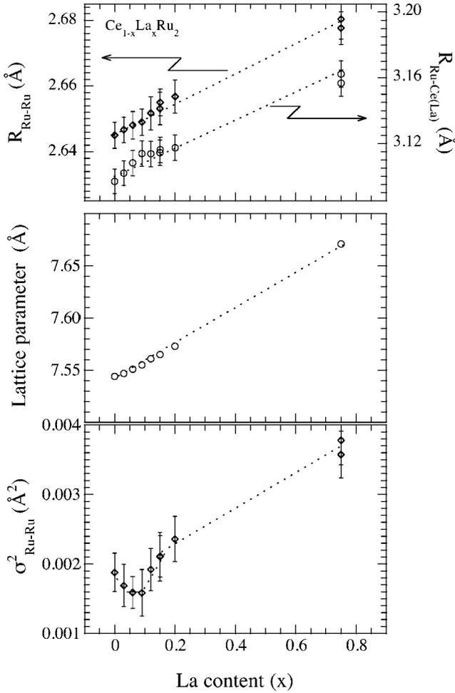
FIG. 4. Ru-Ru and Ru-Ce(La) distances for the  $\text{Ce}_{1-x}\text{La}_x\text{Ru}_2$  system as a function of La concentration showing an almost linear increase (upper), consistent with the variation of the lattice parameter (middle). The Debye-Waller factor of the Ru-Ru pairs is also plotted (lower), revealing a clear change with a small anomaly at low La concentration. The error bars represent the uncertainties estimated by creating correlation maps between different parameters.
