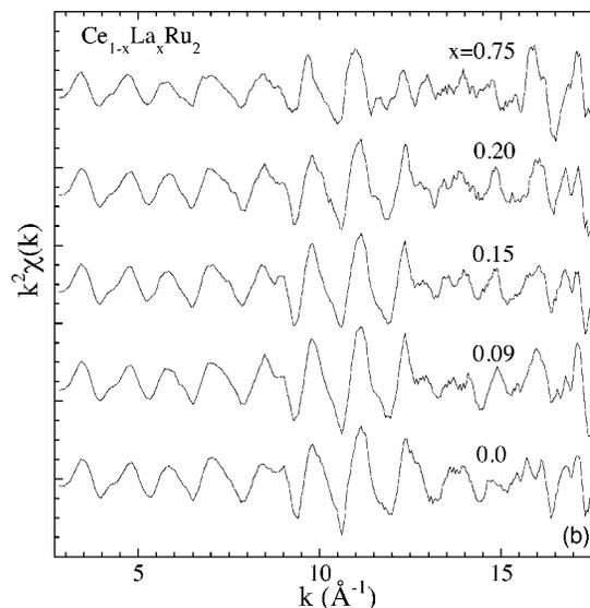
FIG. 1. EXAFS oscillations (multiplied by  $k^2$ ) extracted from the Ru K-edge absorption spectra measured on  $\text{Ce}_{1-x}\text{La}_x\text{Ru}_2$  system for several La concentrations at low temperature (30 K).
