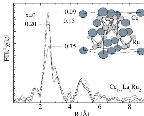
FIG. 2. Fourier transforms of the EXAFS oscillations showing global atomic distribution around the Ru in the  $\text{Ce}_{1-x}\text{La}_x\text{Ru}_2$  system. The Fourier transforms are performed between  $k=3$  and  $17 \text{ \AA}^{-1}$  and not corrected for the phase shifts. The main peak  $\sim 2.5 \text{ \AA}$  is due to Ru-Ru bonds while peak structure  $\sim 3 \text{ \AA}$  represents Ru-Ce(La) bonds. Crystal structure of the  $\text{CeRu}_2$  is shown as an inset.
