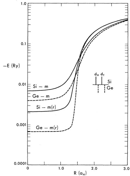
FIG. 1. Ionization energy  $-E$ , in units of the vacuum rydberg, as a function of the cavity radius  $R$ , units of the vacuum Bohr radius  $a_H$  for the cavity models. The estimated cavity radii are  $d_H$  for the hexagonal site and  $d_T$  for the tetrahedral site.
