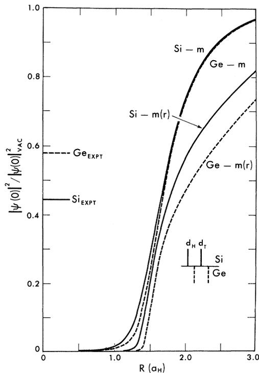
FIG. 2. Probability density ratio  $|\psi(0)|^2/|\psi(0)|_{\text{vac}}^2$  for the cavity models.
