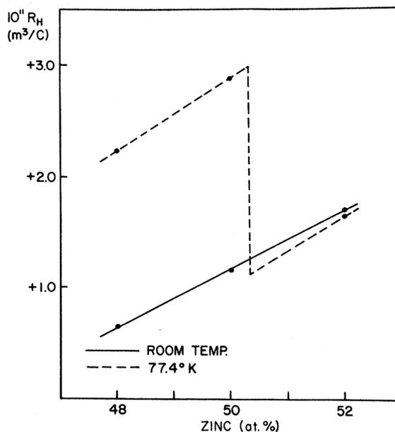
FIG. 1.  $R_H$  of AuZn vs composition at room temperature and at 77.4 °K. Dots are experimental values. The dashed curve connects 77.4 °K points and takes account of transformation (see text).
