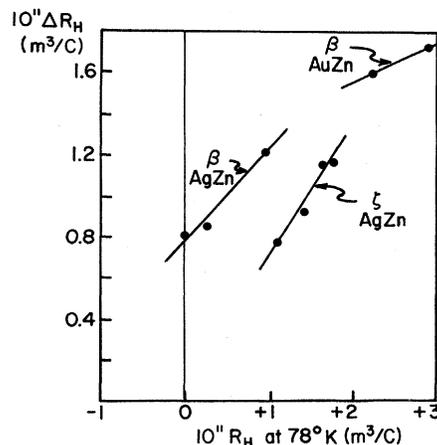
FIG. 3. Differences between room-temperature and liquid-nitrogen-temperature values of the Hall coefficient plotted as a function of  $R_H$  at 77.4 °K for the alloys.
