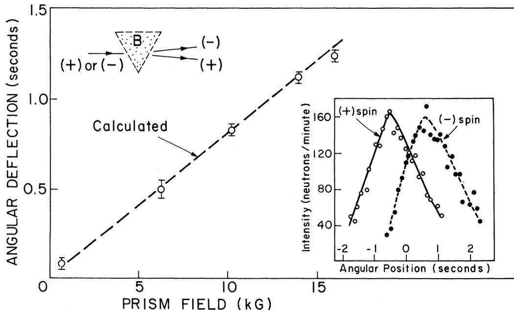
FIG. 1. Typical rocking curves of analyzing crystal (inset) showing deflection of polarized neutron beam (with polarization reversal) upon passage through a 60° prism-shaped magnetic field and deflections measured at different field strengths.
