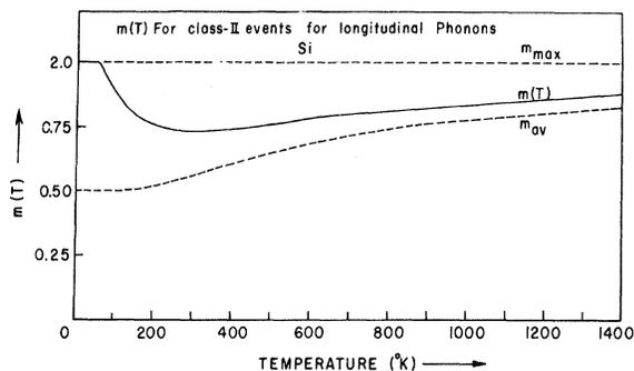
FIG. 4. Temperature dependence of the exponent  $m(T)$  for longitudinal phonons for three-phonon class-II events.  $m_{\max}$  is the maximum limit obtained by Guthrie, and  $m_{\text{av}}$  is the average of upper and lower bounds of Guthrie.  $m_{L,II}(T)$  is the value of exponent  $m(T)$  used in the present calculation.
