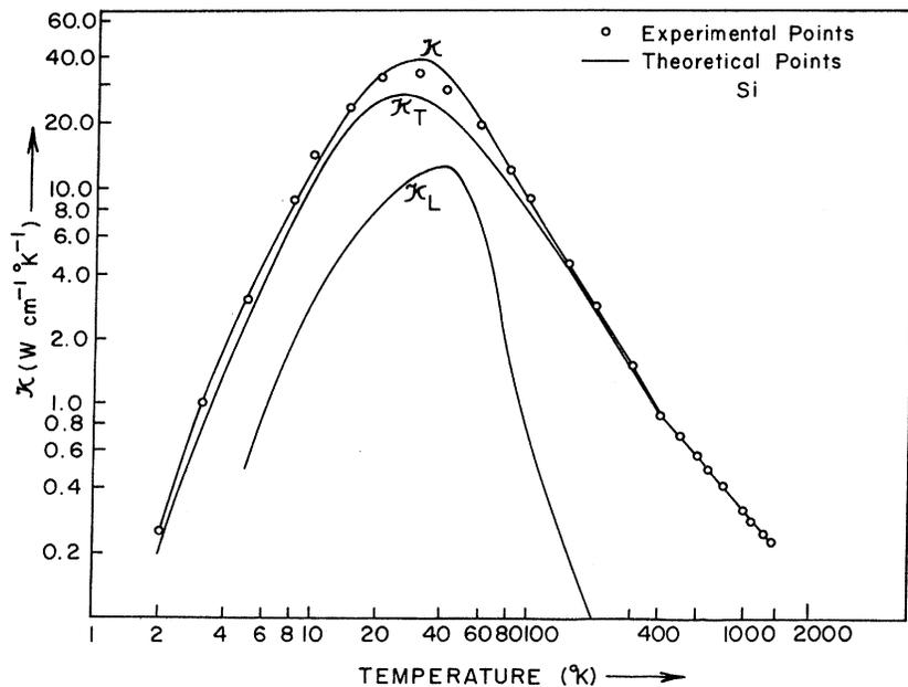
FIG. 1. Comparison of the theoretical values of the phonon conductivity of Si with the experimental values in the temperature range 2–1400 °K.  $\kappa_T$  is the contribution of transverse phonons, and  $\kappa_L$  is the contribution of longitudinal phonons.
