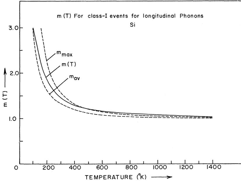
FIG. 3. Temperature dependence of the exponent  $m(T)$  for longitudinal phonons for three-photon class-I events.  $m_{\max}$  is maximum limit obtained by Guthrie, and  $m_{\text{av}}$  is the average of upper and lower bounds of Guthrie.  $m_{L,I}(T)$  is the value of exponent  $m(T)$  used in the present calculation.
