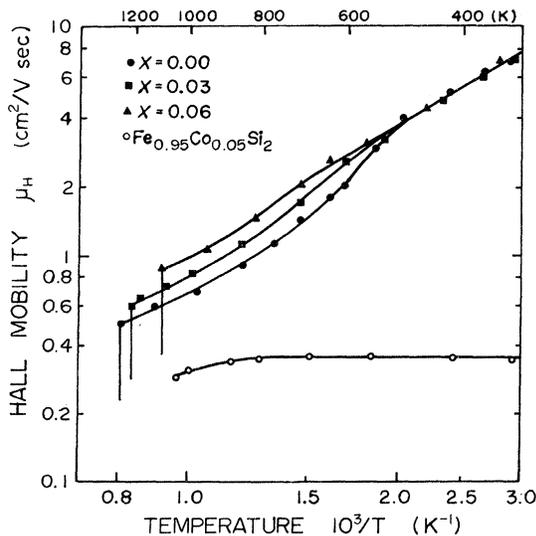
FIG. 3. Temperature dependence of Hall mobility for  $p$ -type  $\text{Fe}_{1-x}\text{Mn}_x\text{Si}_2$ . The open circle is  $n$ -type  $\text{FeSi}_2$ .
