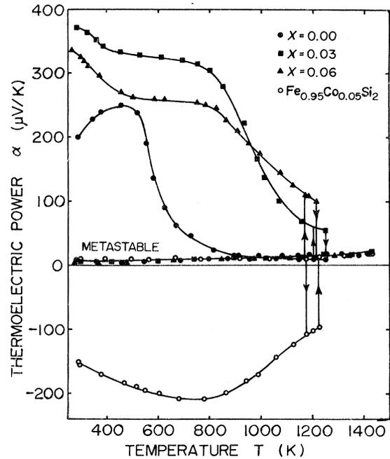
FIG. 2. Temperature dependence of thermoelectric power for  $p$ -type  $\text{Fe}_{1-x}\text{Mn}_x\text{Si}_2$ . Both the heating and cooling transition directions are indicated by arrows, and the open circle is  $p$ -type  $\text{FeSi}_2$ .
