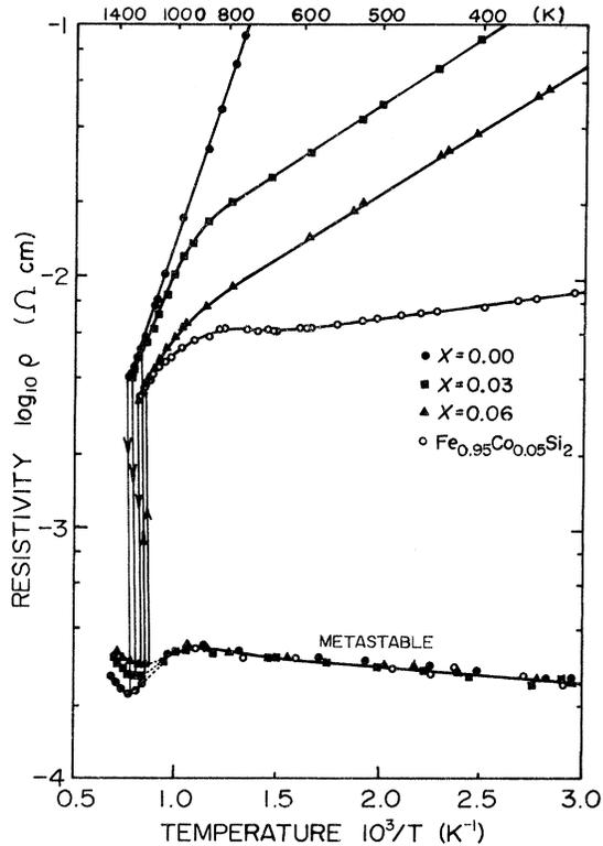
FIG. 1. Temperature dependence of resistivity for  $p$ -type  $\text{Fe}_{1-x}\text{Mn}_x\text{Si}_2$ . Both the heating and cooling transition directions are indicated by arrows, and the open circle is  $n$ -type  $\text{FeSi}_2$ .
