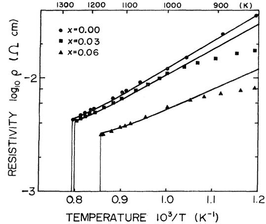
FIG. 4. Temperature dependence of resistivity for  $p$ -type  $\text{Fe}_{1-x}\text{Mn}_x\text{Si}_2$  in the intrinsic region. The solid curves represent the calculated value.
