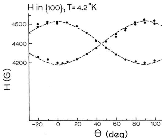
FIG. 3. Angular variation of EPR with  $H$  in  $\{100\}$  plane.  $\nu=9.43$  GHz.
