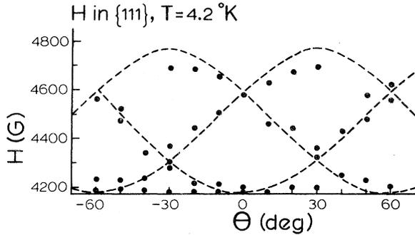
FIG. 4. Angular variation of EPR with  $H$  in  $\{111\}$  plane.  $\nu = 9.43$  GHz.
