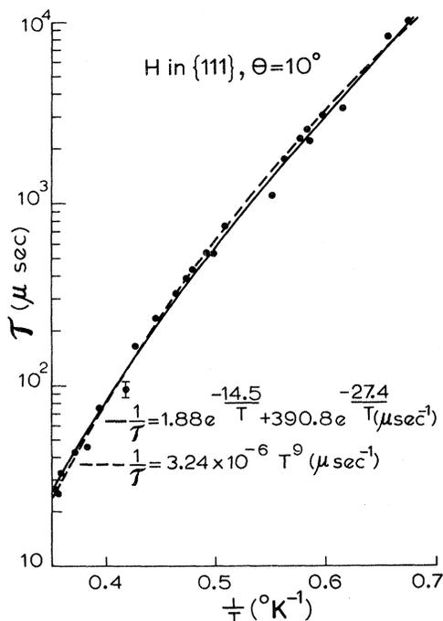
FIG. 2. Arrhenius plot of spin-lattice relaxation results shown in Fig. 1.
