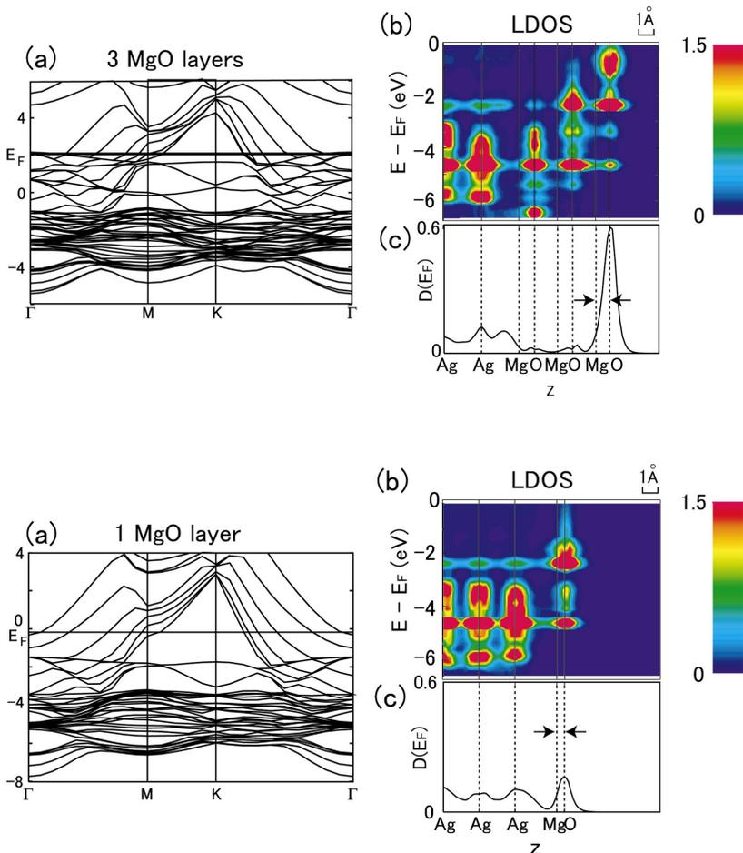
FIG. 3. (Color) The band structure (a), the local density of states (LDOS) integrated over both  $x$  and  $y$  directions displayed as a function of energy and  $z$  ( $\perp$  interface) (b), and the LDOS just at  $E_F$  as a function of  $z$  (c). Vertical dotted lines in (c) represent the optimized positions of atoms, with the separation between the outermost O and Mg indicated with arrows.
