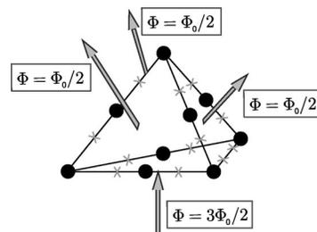
FIG. 1. The superconducting tetrahedron. Each edge consists of a superconducting wire with two Josephson junctions. The tetrahedron is placed in a uniform magnetic field so that the fluxes through the vertical faces are  $\Phi_0/2$  each, while the flux through the horizontal face is  $3\Phi_0/2$ .
