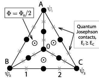
FIG. 2. The equivalent system obtained by tetrahedron projection onto its base. There are two Josephson junctions at each edge. This planar system is placed in the perpendicular magnetic field so that the flux through each of the smaller triangles is half-flux quanta,  $\Phi_0/2$ .
