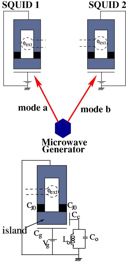
FIG. 1. (Color online) (a) Setup for an entanglement transfer process via the interface between quantum correlated field modes and a pair of charge qubits. Each SQUID is threaded by an external magnetic flux to modulate  $E_J(\phi_{ext})$ . (b) Equivalent circuit for the single SQUID capacitively coupled to a single field mode, modeled as a LC oscillator.
