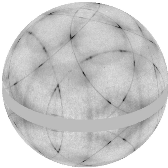
FIG. 7. The (101) pole figure as an intensity chart overlaid on top of a unit sphere. The equatorial band with uniform intensity is the region between 85^\circ < \chi \leq 95^\circ , for which no measured values were available.
