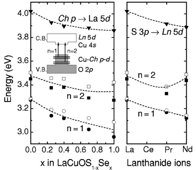
FIG. 4. Absorption peak energies near the band gap edge in (a)  $\text{LaCuOS}_{1-x}\text{Se}_x$  ( $0 \leq x \leq 1$ ) and (b)  $\text{LnCuOS}$  ( $\text{Ln}=\text{La}, \text{Pr}, \text{and Nd}$ ) at 10 K. The central positions between a pair of peaks (open and closed symbols) split by spin-orbit interactions are shown by dashed lines for  $n=1$  and 2. The inset illustrates energy transitions for  $n=1$  and 2.
