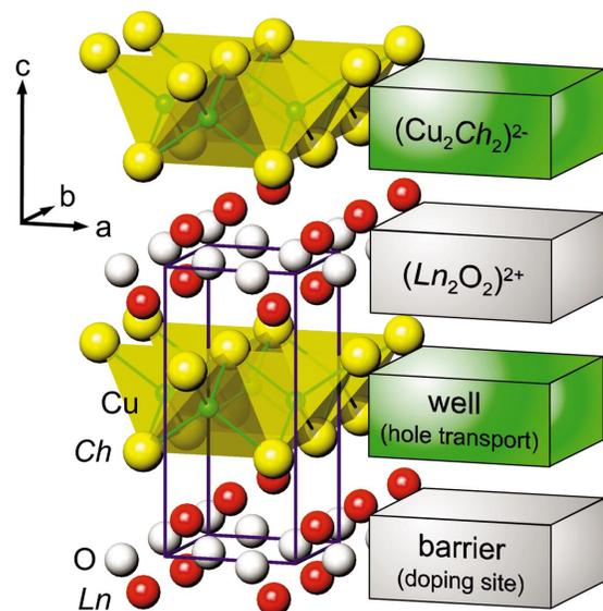
FIG. 1. (Color) Crystal structure of  $LnCuOCh$  (space group:  $P4/nmm$ ).  $(Ln_2O_2)^{2+}$  layers and  $(Cu_2Ch_2)^{2-}$  layers are alternately stacked along the  $c$  axis, forming a MQW structure.
