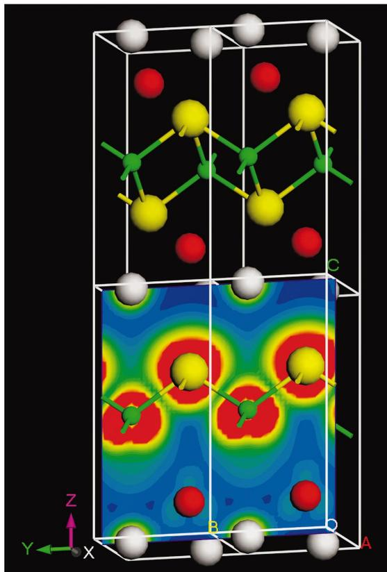
that the VBM orbitals only spread in the  $(\text{Cu}_2\text{S}_2)^{2-}$  layers, which is consistent with the theory that holes are both spatially and energetically confined in the  $(\text{Cu}_2\text{S}_2)^{2-}$  layers. These results demonstrate that the  $(\text{Cu}_2\text{S}_2)^{2-}$  layer works as a well and the  $(\text{La}_2\text{O}_2)^{2+}$  layer serves as a barrier for hole carriers due to the large offset energy at the valence band, forming a QW structure in LaCuOS.
