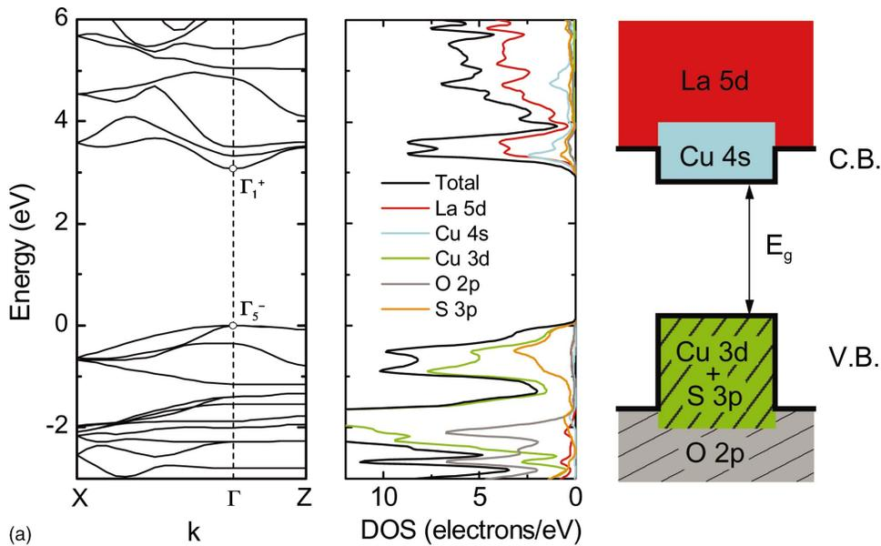
FIG. 2. (Color) (a) Energy band diagram and total/partial DOS of LaCuOS, along with a schematic illustration of the QW structure. (b) Contour plot of the electron density at the energies of around VBM ( $-1.5 \text{ eV} \leq E \leq 0 \text{ eV}$ ), which shows the shape of Cu-S hybridized orbitals.
