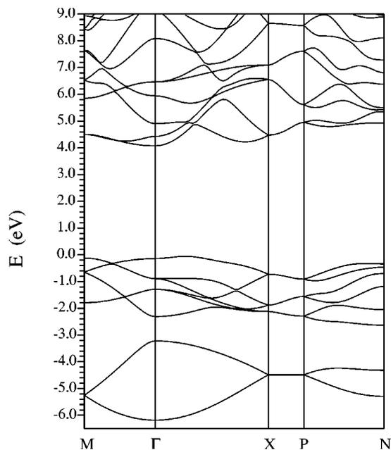
FIG. 2. LDA band structure of  $\text{NaAlH}_4$  with the relaxed crystal structure. The band gap is between a H derived valence band and metal derived conduction bands.
