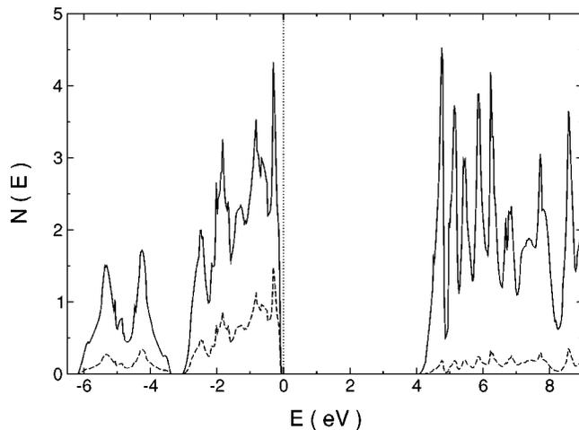
FIG. 3. Electronic density of states and projection onto the H LAPW spheres for  $\text{NaAlH}_4$ , in  $\text{eV}^{-1}$  on a per formula unit basis. Note the ionic nature shown by the very different hydrogen contributions to the valence and conduction bands.
