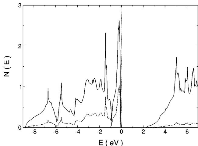
FIG. 5. Electronic density of states and projection onto the H LAPW spheres for  $\text{AlH}_3$ , in  $\text{eV}^{-1}$  on a per formula unit basis, using the relaxed crystal structure. Note the smaller band gap but still ionic nature.
