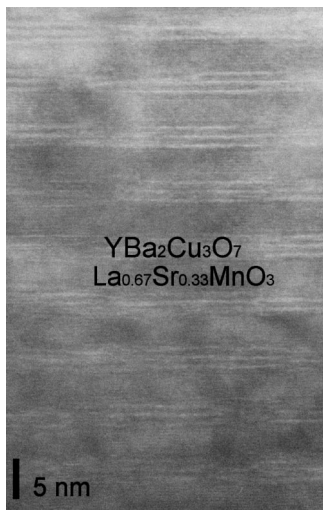
FIG. 2. TEM cross-section image of the [LSMO \times 8 u.c./YBCO \times 3 u.c.] _{16} superlattice.
