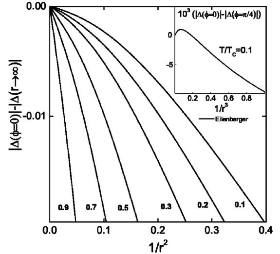
FIG. 2. Behavior of the amplitude of the pairing potential at intermediate distances for  $\phi=0$  and six values of  $T/T_c$  between 0.1 and 0.9. The inset depicts the asymptotical behavior of the difference of the amplitude along 0 and  $\pi/4$  directions,  $|\Delta(\phi=0)| - |\Delta(\phi=\pi/4)|$  at  $T/T_c=0.1$ .
