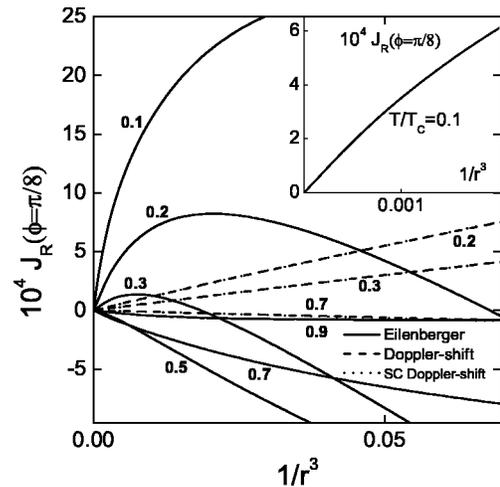
FIG. 7. Asymptotical behavior of the radial component of the supercurrent  $J_R(r)$  at  $\pi/8$  and  $T/T_c=0.1-0.9$  in units of  $-2eN_0v_F\Delta_0$ . The inset demonstrates the  $1/r^3$  relaxation law of the  $J_R(r)$  asymptotic at  $T/T_c=0.1$  on a large scale.
