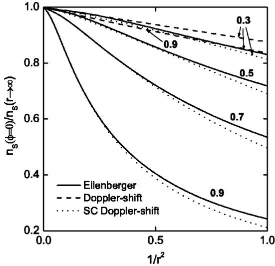
FIG. 5. Asymptotical behavior of the superconducting electron density  $n_s(r)$  normalized to the London value  $n_s(r \rightarrow \infty)$  at long distances at  $\phi=0$  and  $T/T_c=0.3-0.9$ .
