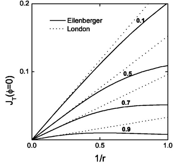
FIG. 4. Asymptotical behavior of the tangential component of the supercurrent  $J_T(r)$  at long distances for  $\phi=0$  and  $T/T_c = 0.1-0.9$  in units of  $-2eN_0v_F\Delta_0$ .
