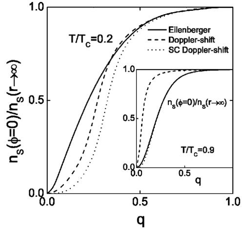
FIG. 6. Superconducting electron density  $n_s(r)$  normalized to the London value  $n_s(r \rightarrow \infty)$  in the whole range of the radius [reduced radius  $q$  is determined by Eq. (8)] at  $\phi=0$  and  $T/T_c=0.2$ . The inset depicts  $n_s(r)/n_s(r \rightarrow \infty)$  at  $\phi=0$  and  $T/T_c=0.9$ .
