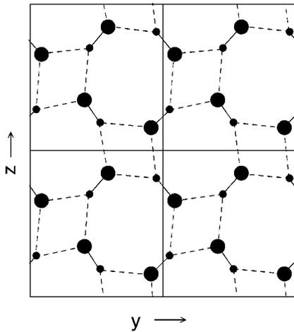
FIG. 1. Schematic representation of the  $\text{HIO}_3$  structure onto the  $yz$  plane. Bigger circles represent  $\text{IO}_3$  groups and the smaller ones hydrogen atoms. Bifurcated hydrogen bonds are represented by solid lines which bifurcate on dashed lines at the hydrogen atoms (after Ref. 15).
