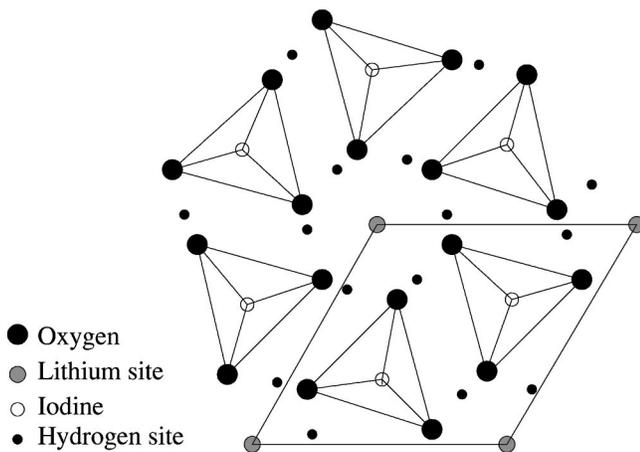
FIG. 2. The crystal structure of  $\text{Li}_{1-x}\text{H}_x\text{IO}_3$  ( $x \approx 0.33$ ) projected onto the  $xy$  plane, according to Ref. 7. In this case, bifurcated bonds are not considered. The protons do not replace the lithium ions, but are randomly distributed in general positions between two oxygen atoms belonging to different iodate groups.
