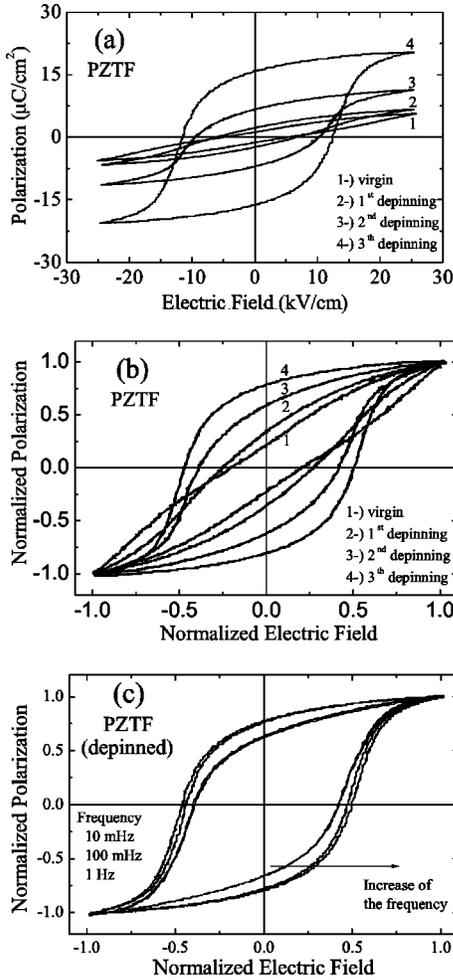
FIG. 7. (a) Hysteresis loop behavior for PZTF measured in the virgin state and during continuous polarization switching. (b) The respective normalized curves ( $P/P_S$  vs  $e/e_{Max}$ ). (c) The frequency dependence of the hysteresis loop for PZTF.
