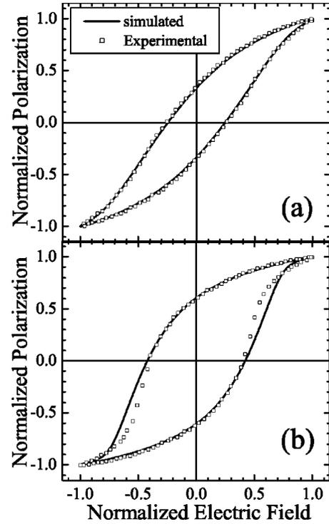
FIG. 8. Comparison of the simulated results with experimental hysteresis loop shown in Fig. 7(b) for (a) second depinning and (b) third depinning processes.
