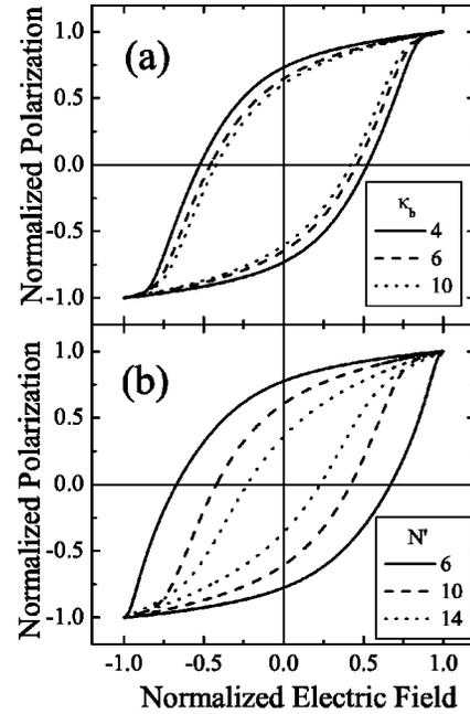
FIG. 4. Simulated hysteresis loop dependence on (a) several values of the interaction coefficient  $\kappa_b$ , and (b) the number of fixed dipoles ( $N'$ ).
