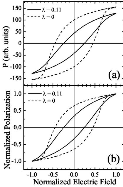
FIG. 3. (a) Dependence of the parameter  $\lambda$  in the hysteresis loop. (b) Same as (a) but for normalized polarization.
