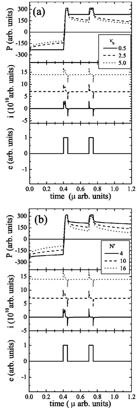
FIG. 2. (a) Response current, polarization, and applied electric pulse dependence with time for several values of the interaction coefficient  $\kappa_b$ . (b) Response current, polarization, and applied electric pulse dependence with time for several values of the fixed dipoles,  $N'$ .
