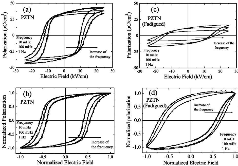
FIG. 6. (a) Hysteresis loop for the PZTN in the virgin state. (b) Respective normalized curves ( $P/P_S$  vs  $e/e_{Max}$ ). (c) Frequency dependence of the hysteresis loop for PZTN in the fatigued state. (d) Respective normalized curves ( $P/P_S$  vs  $e/e_{Max}$ ).
