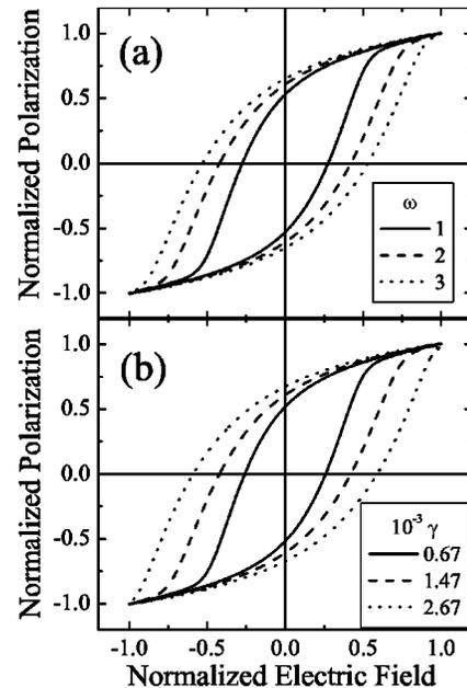
FIG. 5. (a) Frequency dependence of the ferroelectric hysteresis loop. (b) Hysteresis loop dependence on the viscosity coefficient,  $\gamma$ .
