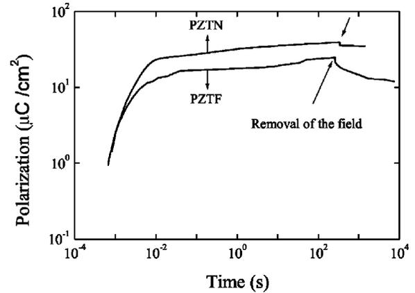
FIG. 9. Time dependence of polarization for PZTN and PZTF during and after the removal of the electric field.
