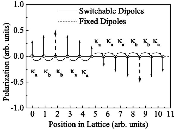
FIG. 1. Schematic representation of the ferroelectric system showing the interaction between the switchable dipole-switchable dipole ( $\kappa_a$ ) and the switchable dipole-fixed dipole ( $\kappa_b$ ).
