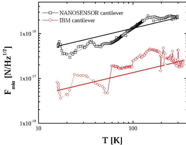
FIG. 5. Minimum detectable force of both cantilevers. The squares and circles are the measured temperature dependences of the sensitivity with variables  $Q^{-1}$  and  $E$  and the lines are the explicit temperature dependence with constant  $Q^{-1}$  and  $E$ .
