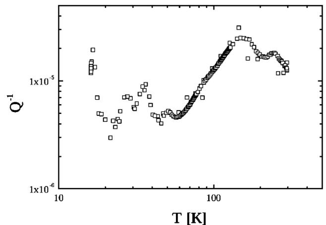
FIG. 4. Measured internal friction of cantilever (b) (Ref. 18). The minimum at 20 K is observed, as predicted by Zener's theory of thermoelastic damping. The peak at  $T = 160$  K is an activation peak and has been observed in other experiments (Refs. 23 and 24).
