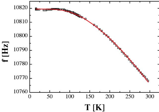
FIG. 2. Measured frequency shift of the cantilever (b) (Ref. 18). The frequency shift is given by the temperature dependence of the Young modulus, as the relative changes of the geometrical dimensions are less than 0.5%. The fitting parameters for the Young modulus give a Debye temperature  $\Theta_D = 634$  K.
