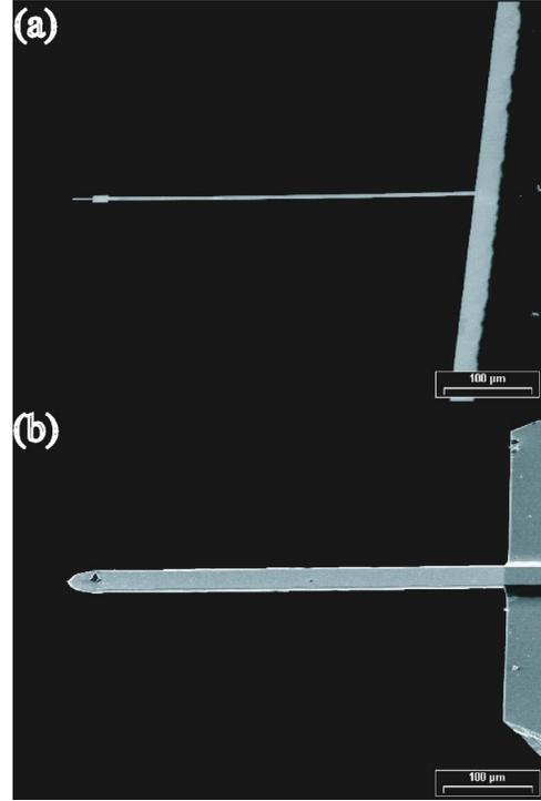
FIG. 1. SEM pictures of the cantilevers. Picture (a) shows the ultrahigh-sensitive cantilever ( $L=454 \mu\text{m}$ ,  $w=4 \mu\text{m}$ ,  $t=0.44 \mu\text{m}$ , and spring constant  $0.1 \times 10^{-3} \text{ N/m}$ ) made by IBM-Rueschlikon and picture (b) the commercially available NANOSENSOR cantilever (Ref. 18), ( $L=450 \mu\text{m}$ ,  $w=45 \mu\text{m}$ ,  $t=2 \mu\text{m}$ , and spring constant  $D=0.176 \text{ N/m}$ ).
