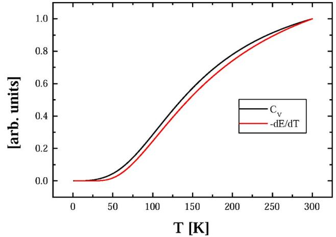
FIG. 3. Comparison of the specific heat capacity  $C_v$  and the negative temperature derivative of Young's modulus  $-dE/dT$ . As required by Nernst's theorem, the temperature deviation of the elastic constants vanishes at 0 K. Both curves are identical if the product of the Grueneisen parameter  $\gamma$  and the Anderson-Grueneisen parameter  $\delta$  is temperature independent and the volume expansion can be neglected.
