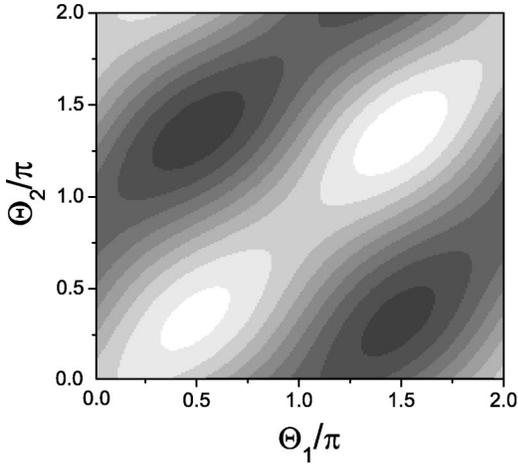
FIG. 2. Contour plot of the interaction term  $W_D$  in the  $(\Theta_1, \Theta_2)$  plane. Two maxima (white regions) and two minima (dark regions) are realized at positions with differences  $\Delta\Theta_1 \approx \pi$  and  $\Delta\Theta_2 \approx \pi$ . Parameter values are given in the text.
