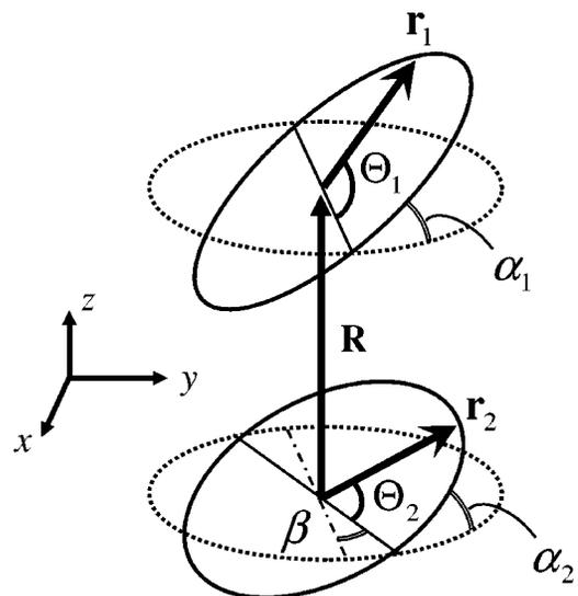
FIG. 1. Schematic configuration of coupled rotors. Each rotor represented by  $\mathbf{r}_1$  and  $\mathbf{r}_2$  rotates along a ring of a radius  $r$ , and carries dipole moment  $qr_{1(2)}$ .
