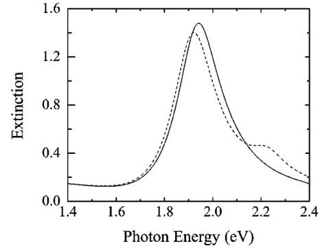
FIG. 2. Extinction spectrum for light incident normally on a square array (lattice constant: 300 nm) of gold spheres (radius: 50 nm) on top of an ITO film (thickness: 140 nm) on a quartz substrate. The solid (dashed) curve is obtained for  $l_{\max} = 1$  ( $l_{\max} = 4$ ).
