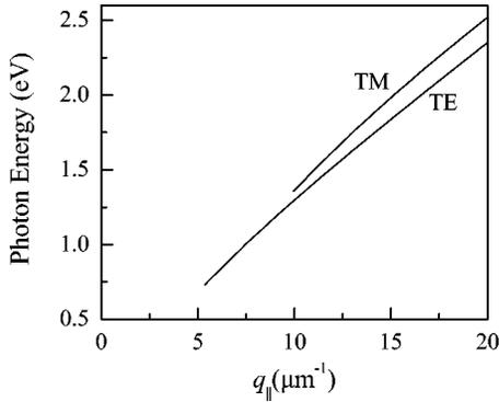
FIG. 1. Dispersion curves of the TE and TM waveguide modes for an ITO film, 140 nm thick, sandwiched between air and quartz.
