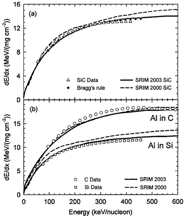
FIG. 2. Measured and predicted (SRIM) stopping powers for Al ions in (a) SiC, along with Bragg values, and (b) C and Si.
