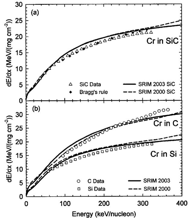
FIG. 3. Measured and predicted (SRIM) stopping powers for Cr ions in (a) SiC, along with Bragg values, and (b) C and Si.
