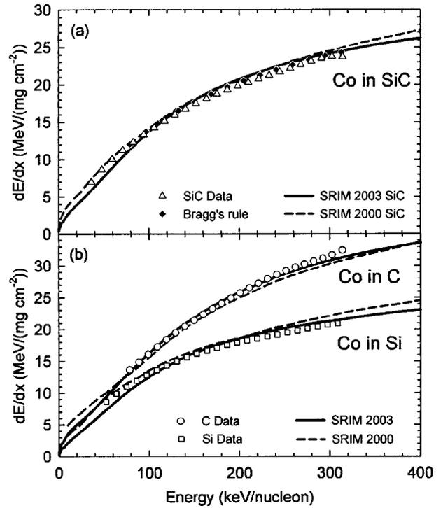
FIG. 5. Measured and predicted (SRIM) stopping powers for Co ions in (a) SiC, along with Bragg values, and (b) C and Si.
