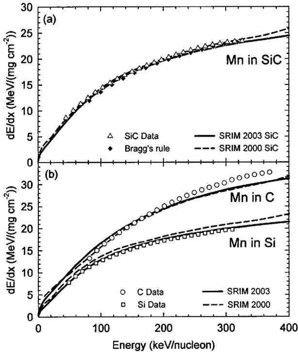
FIG. 4. Measured and predicted (SRIM) stopping powers for Mn ions in (a) SiC, along with Bragg values, and (b) C and Si.
