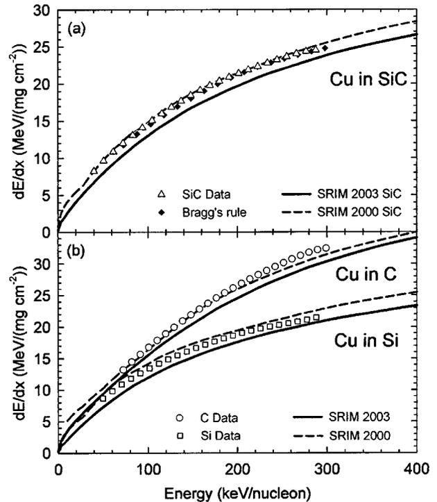
FIG. 6. Measured and predicted (SRIM) stopping powers for Cu ions in (a) SiC, along with Bragg values, and (b) C and Si.
