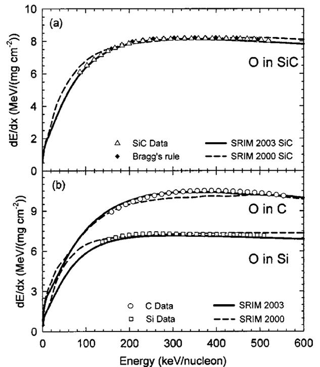
FIG. 1. Measured and predicted (SRIM) stopping powers for O ions in (a) SiC, along with Bragg values, and (b) C and Si.
