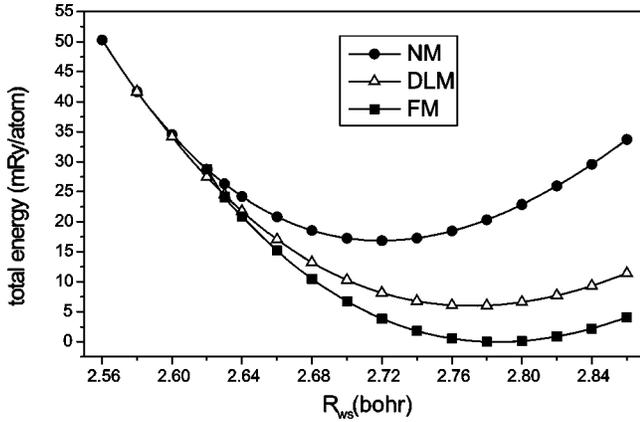
FIG. 1. Total energy as a function of the volume given in terms of the Wigner-Seitz radius. NM: nonmagnetic. FM: ferromagnetic. DLM: disordered local moment.
