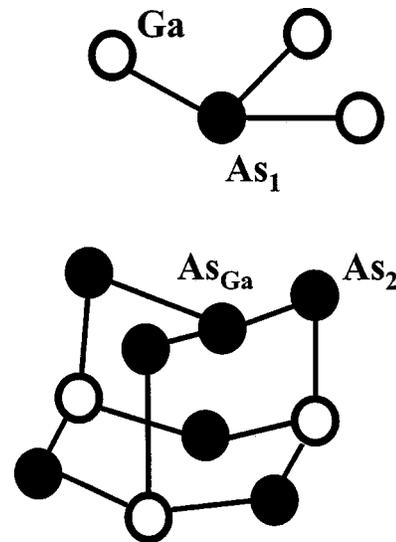
FIG. 1. Metastable configuration for the neutral state (EL2M) of the As-antisite defect in GaAs. This configuration with a smaller  $\text{As}_1 - \text{As}_{\text{Ga}}$  separation is the *ground state* for negatively charged states of the As antisite in *n*-type GaAs when the Fermi level lies at the conduction band edge or higher.
