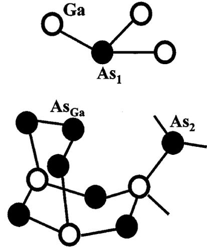
FIG. 2. An alternative low energy structure for the  $-2$  charged state of the As-antisite defect in GaAs is shown. This structure is degenerate with that shown in Fig. 1 for the  $-2$  state.
