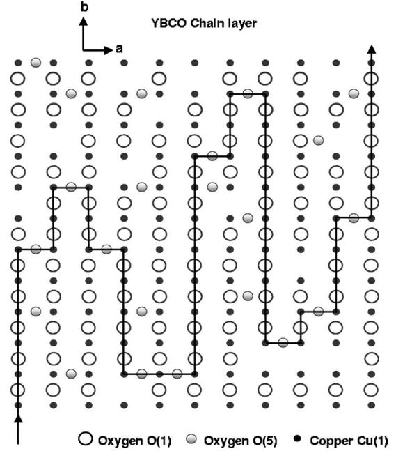
FIG. 8. Representation of the proposed local structure of the chain layer. Chain oxygen O(1) ions are represented by open circles, interchain oxygen O(5) by shaded circles, and copper ions by black dots. Black solid line represents a possible zigzag path of the transport current through O(5) sites in the chain layer.
