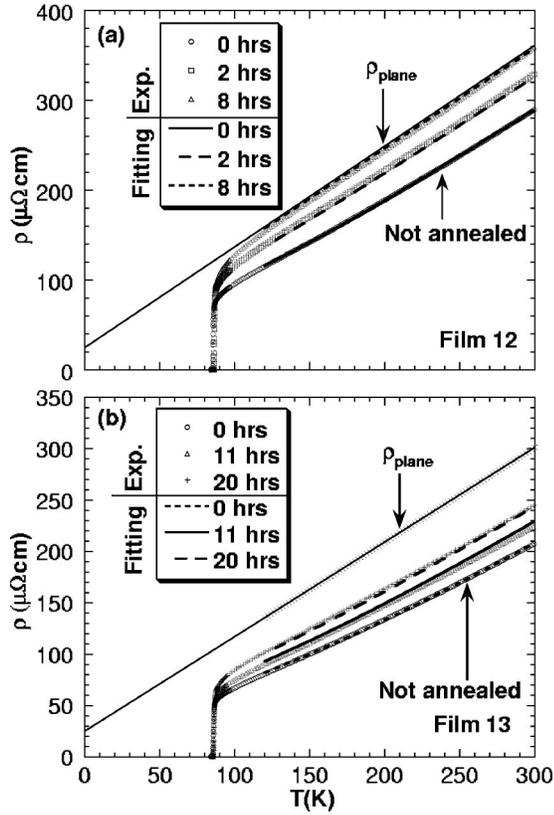
FIG. 9. Experimental data and theoretical fitting curve obtained between 120 and 300 K, using the proposed model described in the text, for  $\rho_{ab}(t, T)$  measured in slightly underdoped films 12 and 13. The assumed resistivity of the planes  $\rho_{planes}(T)$  in Eq. (9) is represented by the solid line marked  $\rho_{plane}$  at temperatures between 120 and 300 K.
