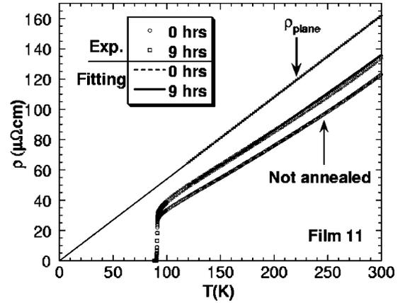
FIG. 10. Experimental data and theoretical fitting curves obtained between 120 and 300 K, using the proposed model described in the text, for  $\rho_{ab}(t, T)$  measured in the optimally doped film 11. The assumed resistivity of the planes  $\rho_{planes}(T)$  in Eq. (9) is represented by the solid line marked  $\rho_{plane}$  at temperatures between 120 and 300 K.
