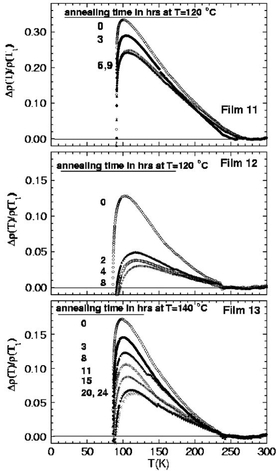
FIG. 6. Upward deviation of  $\rho_{ab}(T)$  (measured for films 11, 12, and 13) from the linear temperature dependence of resistivity  $\rho(T)$ , defined as  $\Delta\rho(T)/\rho(T_1)=[\rho_{ab}(T)-\rho(T)]/\rho_{ab}(T_1)$ , where  $T_1$  is the temperature at which the maximum upward deviation of  $\rho_{ab}(T)$  from a linear  $\rho(T)$  occurs. Note the saturation of  $\Delta\rho(T)/\rho(T_1)$  after annealing times of 6 h for film 11, and 20 h for film 13, respectively.
