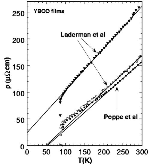
FIG. 2. Temperature dependence of the in-plane resistivity  $\rho_{ab}$  measured in  $c$ -axis oriented epitaxial YBCO thin films. The data indicate that films with low resistivity exhibit a deviation from the linear temperature dependence at temperatures below  $\approx 230$  K (Refs. 9,10).
