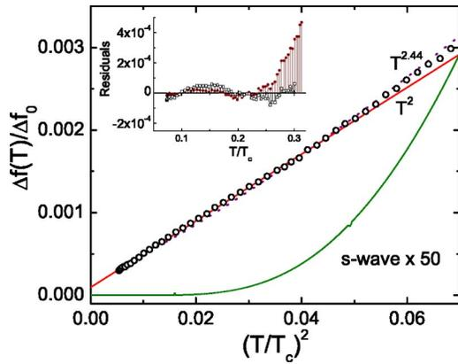
FIG. 3. Penetration depth plotted versus  $T^2$  compared to a standard  $s$ -wave curve. The fit to a pure  $T^2$  behavior is shown by solid line. The fit to  $T^n$  with  $n$  as a free parameter is shown by dotted line. Inset: residuals for fit with  $n=2$  (solid symbols) compared to the residuals of  $n=2.44$  fit. The vertical scale of the inset is the same as in the inset of Fig. 2 for comparison.
