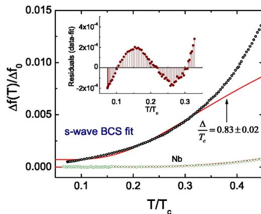
FIG. 2. Upper curve: Best *s*-wave BCS fit for  $\text{MgCNi}_3$  using a standard expression (described in the text) with  $\Delta(0)/T_c$  as a free parameter. The lower curve shows Nb sample and a standard BCS fit. Inset: residuals, *Data - Fit*, for the best *s*-wave BCS fit, which yields  $\Delta(0)/T_c = 0.83 \pm 0.02$ .
