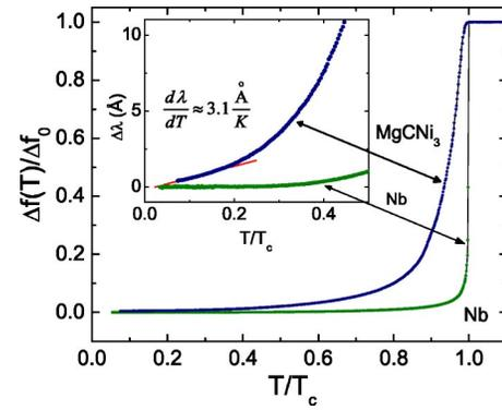
FIG. 1. Magnetic penetration depth measured in zero external field in  $\text{MgCNi}_3$  (upper curves) compared to polycrystalline Nb foil (lower curves). The inset shows actual penetration depth values at low temperatures.
