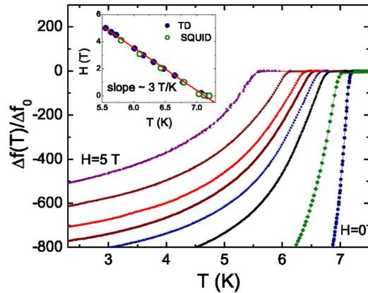
FIG. 4.  $\lambda(T)$  measured at different values of the external dc magnetic field, from  $H=0$  to  $H=5$  T. The inset shows onset of superconductivity in tunnel diode measurements (closed symbols) compared to superconducting quantum interference device (SQUID) magnetometer measurements (open symbols).
