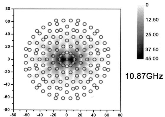
FIG. 3. The distribution of electric field at three frequencies which correspond to the peaks within the low-transmission region of Fig. 2.
