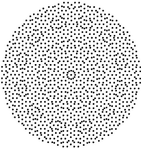
FIG. 1. Two-dimensional dodecagonal quasiperiodic photonic crystal.
