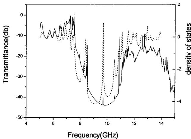
FIG. 2. Total energy flow (solid line) and the density of states (dashed line) of a dodecagonal QPC constructed with 145 cylinders.
