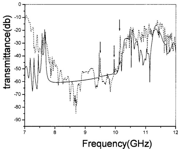
FIG. 4. The measured (dotted line) and calculated (solid line) transmittance of the defect-free dodecagonal quasiperiodic photonic crystal.
