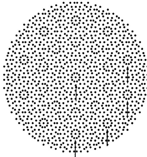
FIG. 5. Two-dimensional decagonal quasiperiodic photonic crystal. The arrows indicate the identical regions in decagonal QPC.
