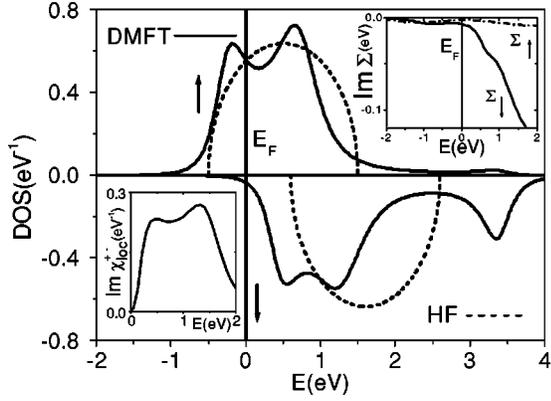
FIG. 1. Density of states for HMF in the Hartree-Fock (HF) approximation (dashed line) and the QMC solution of DMFT problem for the semicircular model (solid line) with the band width  $W = 2$  eV, Coulomb interaction  $U = 2$  eV, spin splitting  $\Delta = 0.5$  eV, chemical potential  $\mu = -1.5$  eV, and temperature  $T = 0.25$  eV. Insets: imaginary part of the local spin-flip susceptibility (left) and the spin-resolved self-energy (right).
