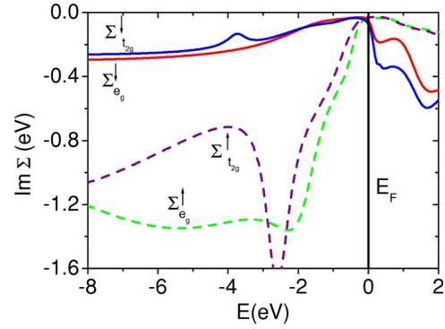
FIG. 4. The imaginary part of self-energies  $\text{Im}\Sigma_d^\uparrow$  for  $t_{2g}$  (solid line) and  $e_g$  (dotted line) and  $\text{Im}\Sigma_d^\downarrow$  for  $t_{2g}$  (dashed line) and  $e_g$  (dashed dotted line), respectively.
