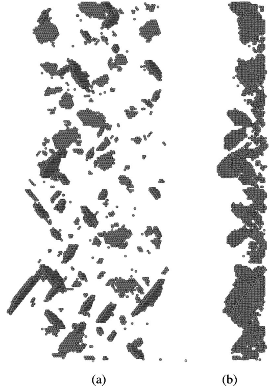
FIG. 4. Defect nucleation at u_p = 2.3\sqrt{\epsilon/m} . (a) and (b) are tilted around the (010) axis, (b) is a side view of the shock (the propagation occurs towards the right).
