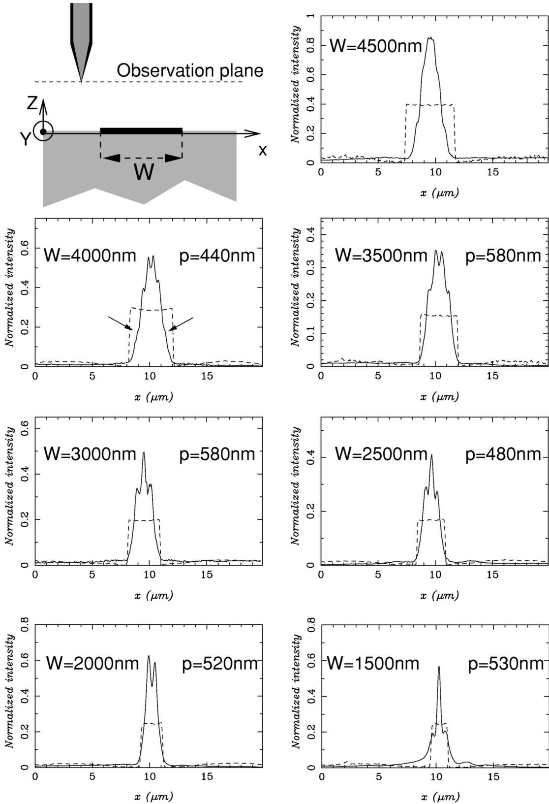
FIG. 3. Over the various stripes, cross cuts of the near-field intensity distribution recorded at a constant height. The dashed lines are guides to the eye, indicating the stripe widths (see text). The values of  $p$  give the distances between the peaks.
