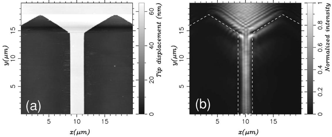
FIG. 6. (a) AFM and (b) PSTM images of the junction between the extended thin film and the 2.5- $\mu\text{m}$ -wide stripe.
