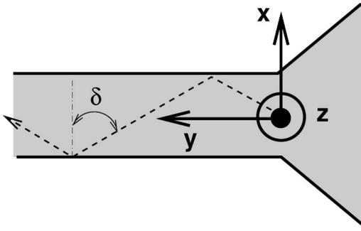
FIG. 4. Schematic view of a SP multireflection on the edges of a metal stripe.
