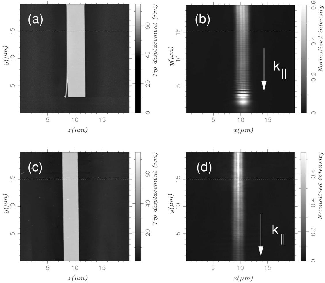
FIG. 2. [(a) and (c)] AFM and [(b) and (d)] PSTM images of two stripes:  $w=3.5 \mu\text{m}$  in (a) and (b) while  $w=2.5 \mu\text{m}$  in (c) and (d). The intensity scales of the PSTM images are normalized independently of each other: for each sample, the unit intensity is defined as the highest intensity detected above the stripe. For the sake of better visualization, the scale has been saturated to 0.6 in (b) and to 0.75 in (d).
