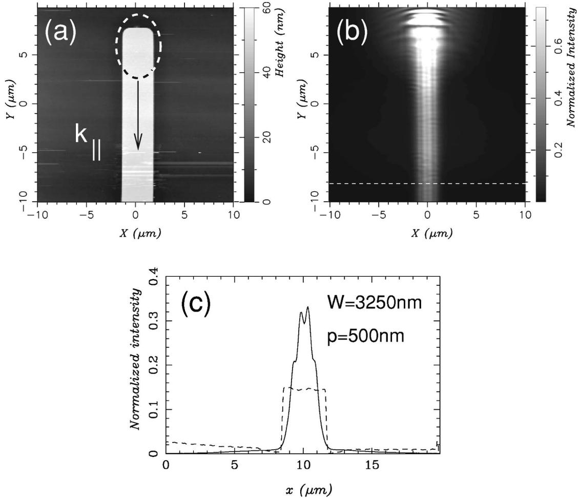
FIG. 7. (a) Topographic image of a MS with a width  $W=3.25 \mu\text{m}$  and thickness  $t=55 \text{ nm}$ . (b) PSTM image recorded when the input end of the MS is directly illuminated by the incident spot. The average angle of incidence is equal to  $\theta_{SP}$  and the plane of incidence is parallel to the  $y$  axis. (c) Cross cut of (b) taken along the white dashed line. The period of the longitudinal oscillations is 500 nm.
