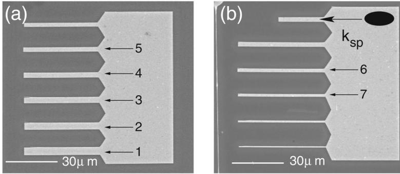
FIG. 1. Scanning electron microscope images of 55-nm-thick gold stripes. The widths of the stripes, labeled from 1 to 7, ranges from 4.5 to 1.5  $\mu\text{m}$  by steps of 0.5  $\mu\text{m}$ . A focused laser beam ( $\lambda = 800$  nm) is incident from the substrate at an angle suitable to excite the SP on the extended thin film. An example of the location of the resulting spot is schematically shown in the upper part of (b).
