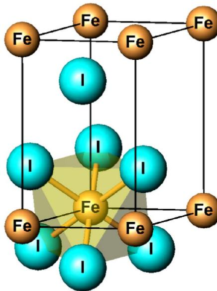
FIG. 1. Crystal structure of  $\text{FeI}_2$ , showing the hexagonal I-Fe-I sandwich layers.  $\text{FeI}_6$  octahedron is shown to indicate the orientation, which has one face perpendicular to the hexagonal  $c$  axis.
