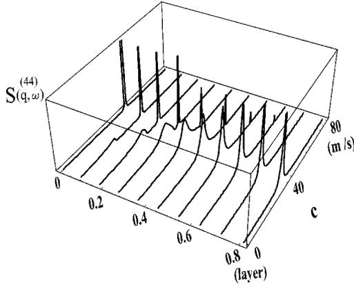
FIG. 2. The Dynamical structure function  $S^{(44)}(q, \omega)$  for a fixed wave number  $q$  is plotted as a function of the concentration of  ${}^3\text{He}$  and the velocity of excitation. The third sound evolves to the lower branch, and the spectral weight  $S^{(44)}(q, \omega)$  is broadened as concentration of the  ${}^3\text{He}$  quasiparticle increase. Parameters  $u_i$ ,  $d$ , and  $h_4$  are the same as in Fig. 1.
