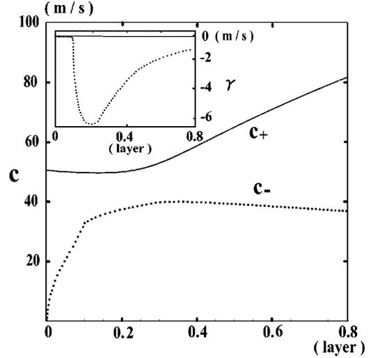
FIG. 1. Real and imaginary parts (inset) of the spectrum are plotted with  $\omega/q = c + i\gamma$  as functions of the concentration of the  $^3\text{He}$ . Here we fix the thickness of  $^4\text{He}$  films to  $d = 25.3 \mu\text{mol}/\text{m}^2$  and  $h_4 = 25.8 \mu\text{mol}/\text{m}^2$ , and the graphite sheet is modeled as a substrate.
