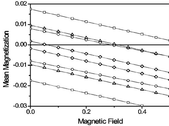
FIG. 3. Mean magnetizations of both paramagnetic (upper curve) and diamagnetic (lower curve) solutions for Josephson junction mixed arrays. For all curves  $\alpha=0.25$  and  $\beta=0.04$ :  $\circ$   $N=63$  with a single  $\pi$ -loop;  $\diamond$   $N=255$  with 15  $\pi$  loops and one odd paramagnetic half flux quantum;  $\triangle$   $N=255$ , with 15  $\pi$  loops and ten paramagnetic half flux quanta;  $\square$   $N=255$ , with 15  $\pi$  loops and 12 paramagnetic half flux quanta.
