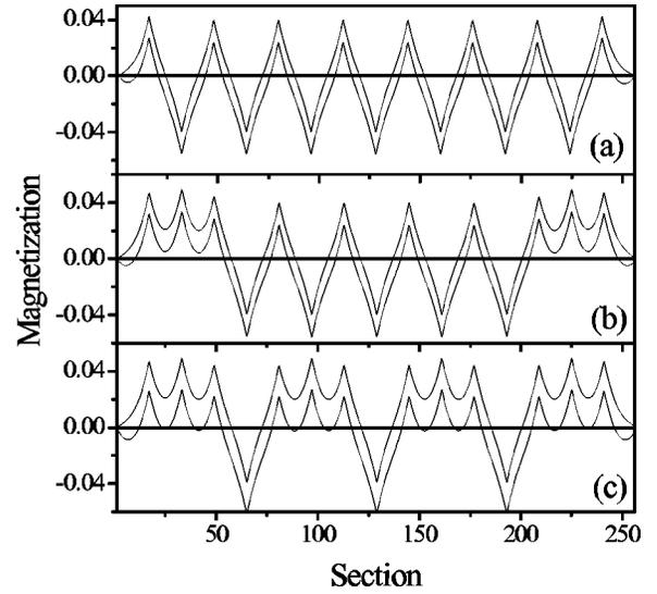
FIG. 4. Simulated magnetization of a  $N=255$  Josephson junction 15  $\pi$ -loop array with  $\beta_L=0.04$  and  $\alpha=0.25$ : (a) Solution with one unpaired paramagnetic half flux quantum; top curve  $\eta=0$ ; bottom curve  $\eta=0.1$ . (b) Solution with ten paramagnetic half flux quanta; top curve  $\eta=0$ , bottom curve  $\eta=0.5$ ; (c) Solution with 12 paramagnetic half flux quanta; top curve  $\eta=0$  bottom curve  $\eta=0.7$ .
