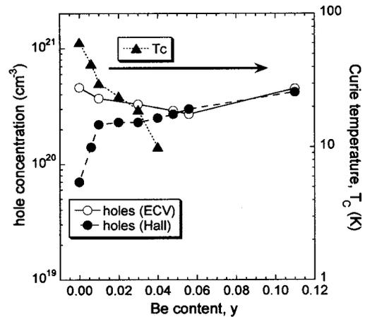
FIG. 3. Hole concentrations determined by ECV and Hall measurements and the Curie temperatures  $T_C$  for as-grown  $Ga_{1-x-y}Mn_xBe_yAs$  films with increasing Be content  $y$ .
