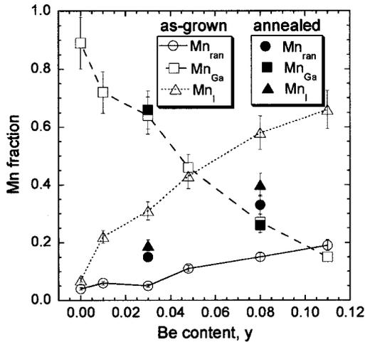
FIG. 2. Fractions of Mn atoms at the various sites—substitutional ( $Mn_{Ga}$ ), interstitial ( $Mn_I$ ), and in random-cluster form ( $Mn_{ran}$ )—as measured from the angular scans shown in Fig. 1. The Mn fractions for the sample with  $y \sim 0.03$  and  $0.08$  annealed at  $280^\circ\text{C}$  for 1 h are also shown as solid symbols.
