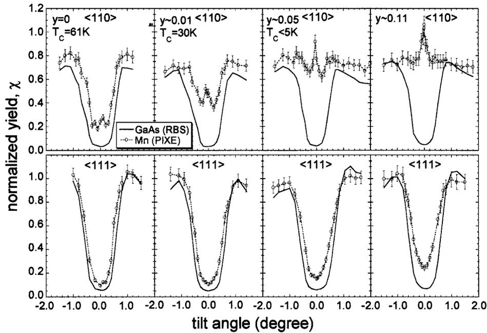
FIG. 1. Angular scans about the  $\langle 110 \rangle$  and  $\langle 111 \rangle$  axes for undoped and Be-doped  $\text{Ga}_{1-x}\text{Mn}_x\text{As}$  samples. The  $\langle 110 \rangle$  angular scans are taken along the  $\{110\}$  planar channel.
